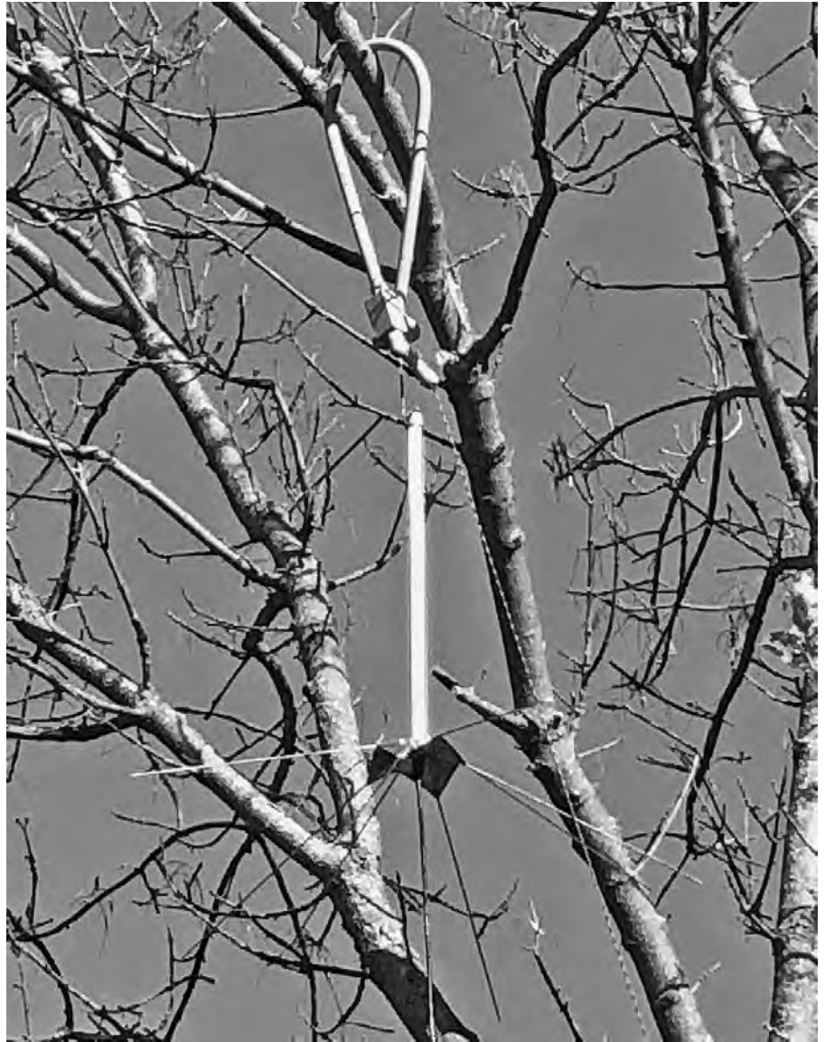
Figure 4 — The tree branch gadget locked in place and supporting a 2-m band quarter-wavelength vertical antenna.
