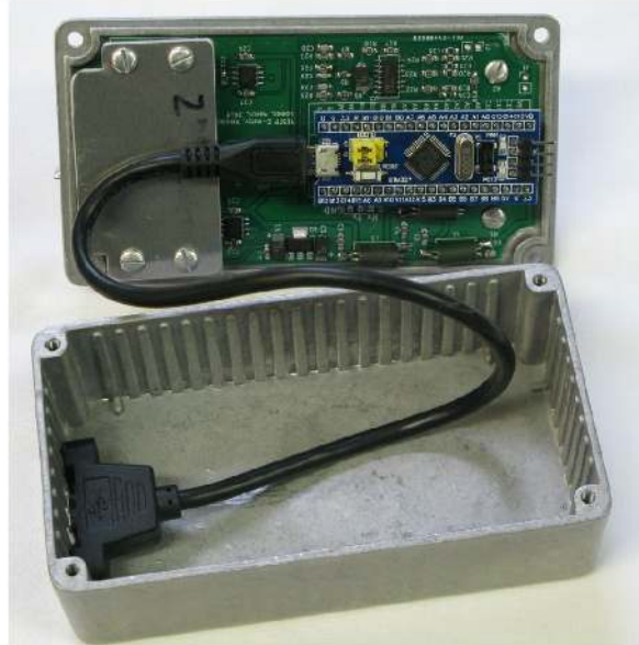
Figure 4 — The PCB fits inside the lid of a die-cast box.
