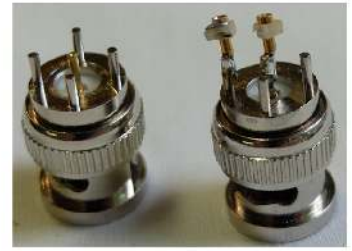
Figure 12 — BNC test connector (left) found on eBay, and on (right) a homebrew connector, both with spacing to match HC-49 crystals.
