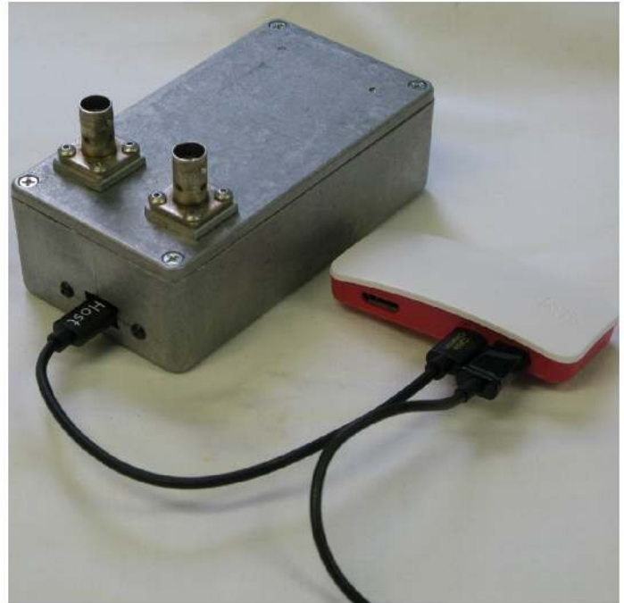
Figure 15 — Impedance meter with the Raspberry Pi Zero W attached.
