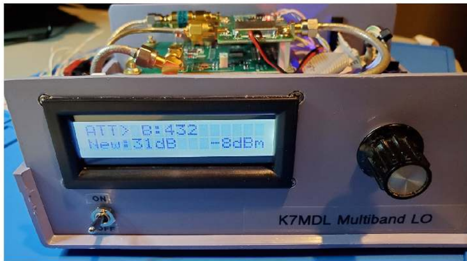
Figure 6 — Attenuation Config Menu shows 432 MHz band with 31 dB attenuation setting and -8 dBm measured output.
