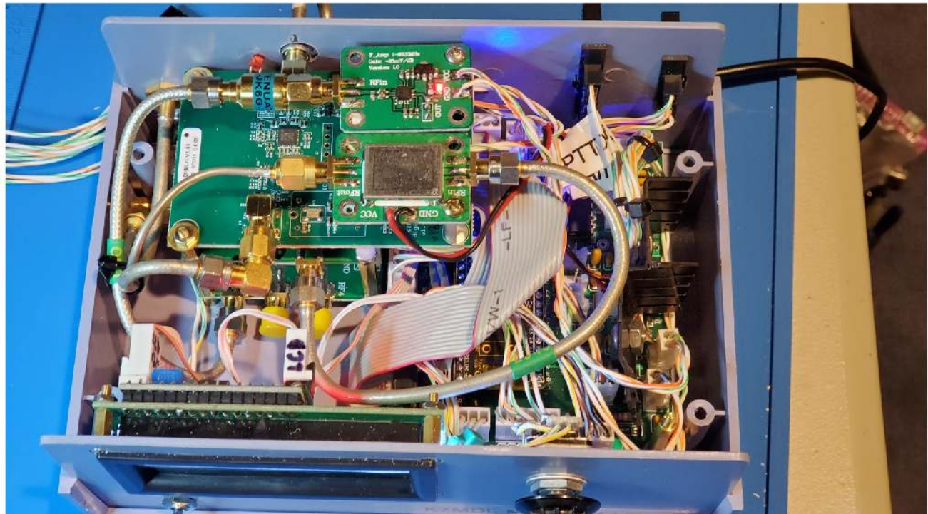
Figure 3 —The log power detector is at the top center, the wideband amplifier is at the top of the lower position. Under that is a stack of top to bottom: the PLL, the attenuator, and the RF switch.
