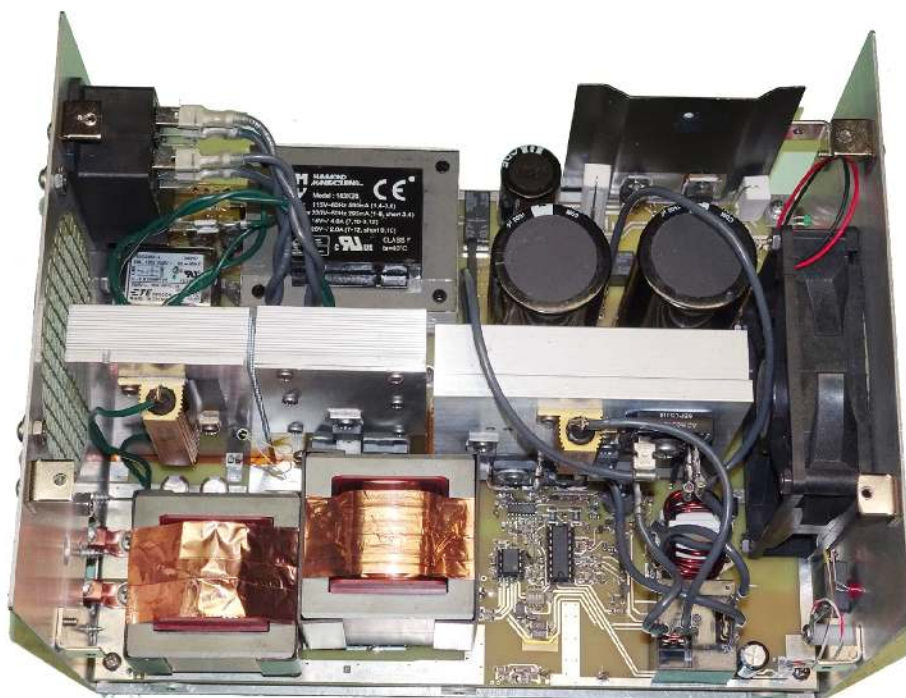
Figure 2 — Top view of the completed PC board installed on the chassis.
