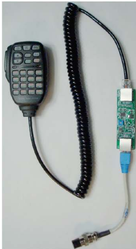
Figure 2 — The DTMF adapter assembly operates as a dongle. The final assembly would be covered by a 3D printed enclosure or by a large-diameter heat shrink sleeve.
