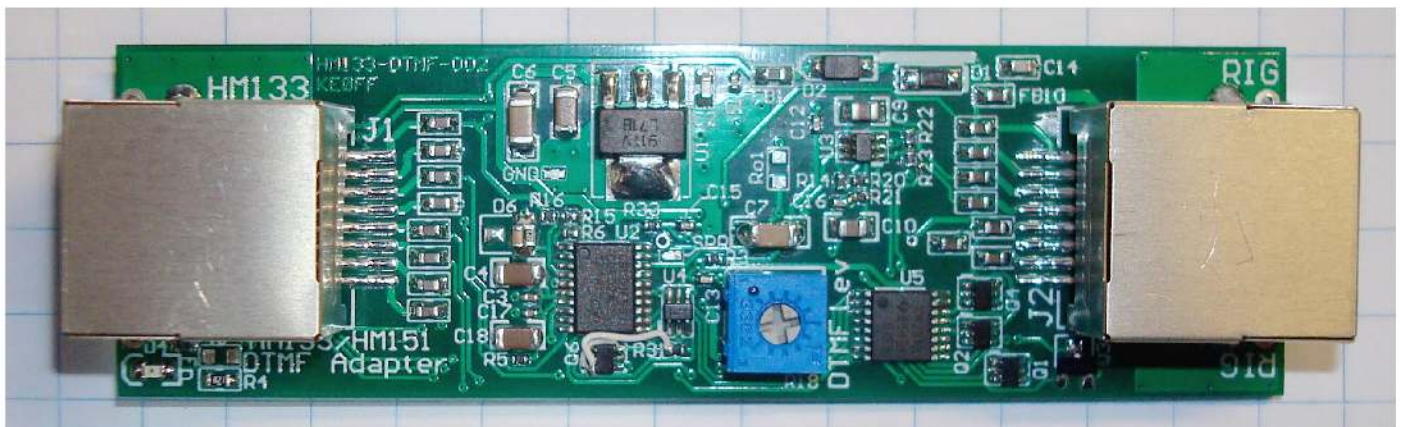
Figure 1 — The HM-133 DTMF adapter assembly.
