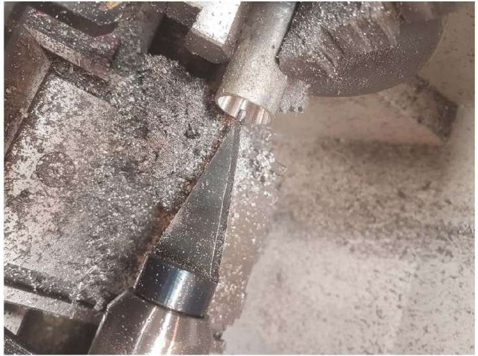
Figure 7 — Tool used to bore out the internal tapered hole in the conical horns.
