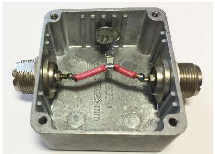
Figure 5 — This 80 m tuner uses a single capacitor.
