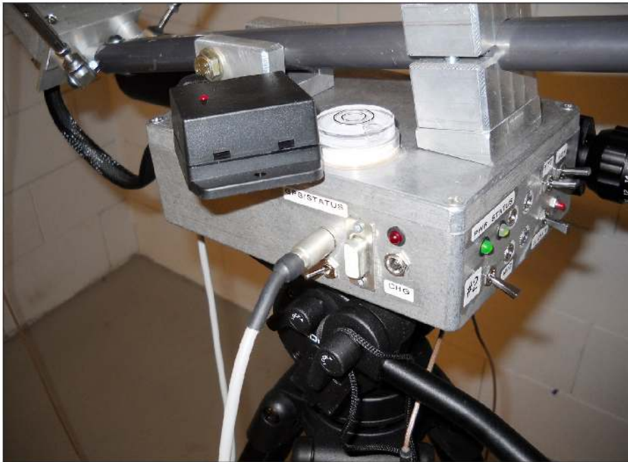
Figure 11 — The control box (bare metal) with GPS unit (black) atop.
