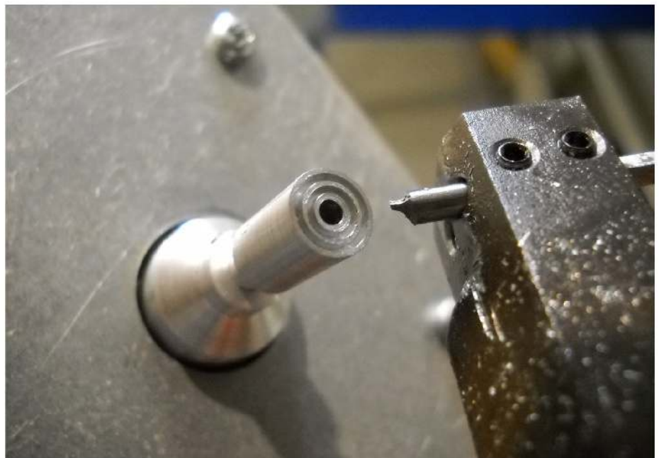
Figure 8 — Machining of the Chaparral feed uses a special tool made from a broken tap.
