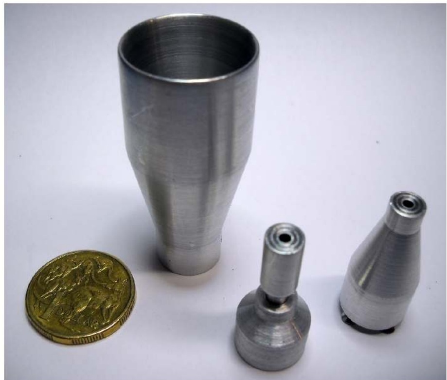
Figure 9 — A horn antenna, and adjustable and fixed feeds.
