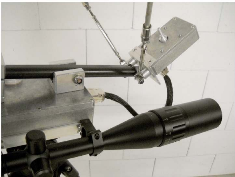
Figure 10 — The feed point and the telescopic sight.
