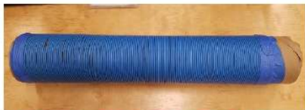
Figure 2 — The actual winding of wire onto the pole was from a 3-inch diameter cardboard mailing tube pre-wound with 151 feet of wire.
