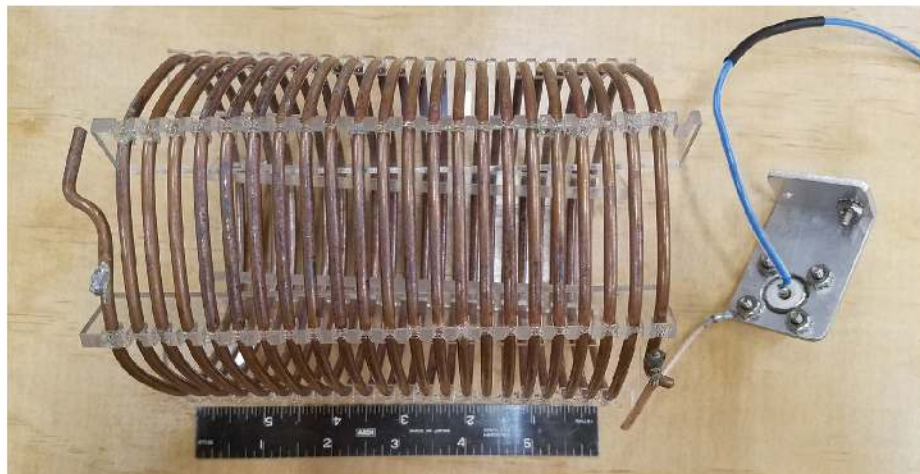
Figure 3 — The radial loading coil design uses six 1/8" thick by 1/2" deep acrylic coil supports.
