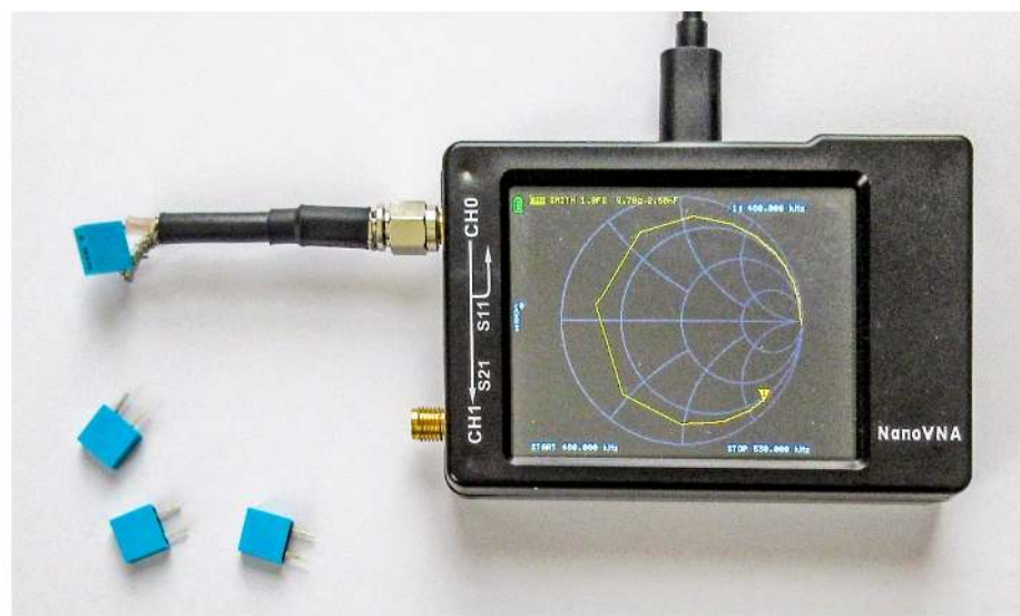
Figure 2 — Test circuit for measuring S11.
