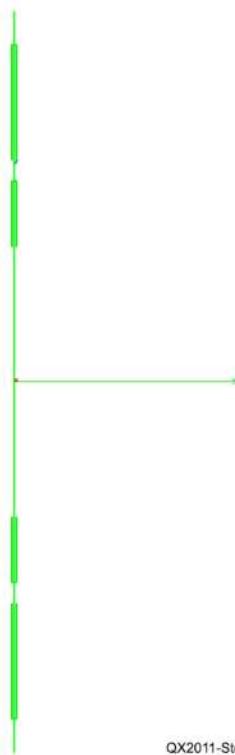
Figure 2 — A triband Extended Double Zepp (EDZ) antenna model.
