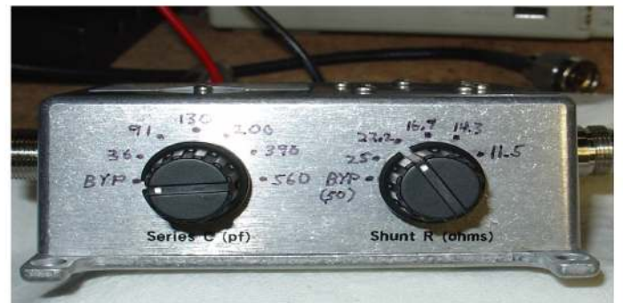
Figure 13 — Front view of the antenna simulator test box.
