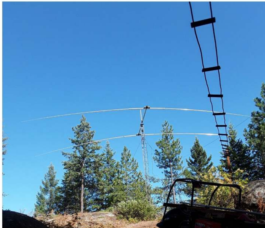
Figure 2 — The W7SX array. The open-wire transmission line is seen on the right.
