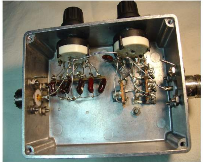
Figure 11 — Internal view of antenna modeling fixture.
