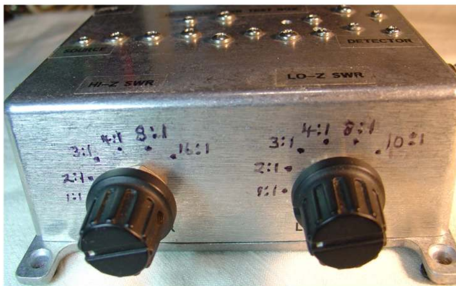
Figure 2 — SWR Test box front panel.
