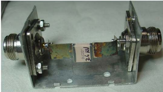
Figure 15 — Internal view of the SWR degradation box.
