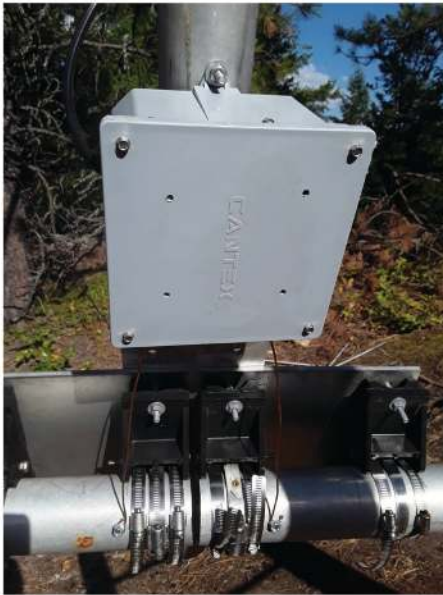
Figure 3 — An electrical box attached to the 3" boom houses the reactive components and relays.
