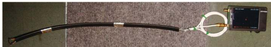
Figure 6 — 150\ \Omega load matched to 50\ \Omega on 432\ \text{MHz} .
