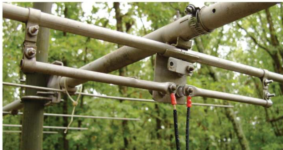
Figure 7 — T match connection to twin lead on 2-meter antenna.
