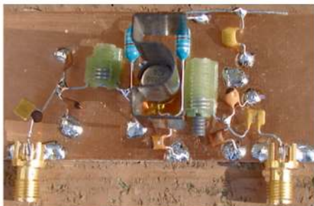
Figure 1 — The small RF power amplifier test set using a 2N3866, center with attached heat sink. RF input is on the left, and output is on the right.
