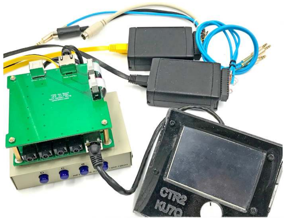
Figure 1 — The basic multi-radio CTR2 system consists of the HMI board, an RJ45 adapter board, a color remote display, a manual RJ45 switch, and a couple of radio I/O modules.
