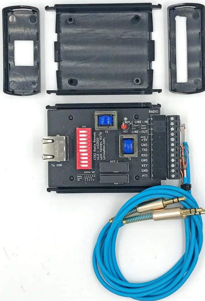
Figure 10 — The radio I/O module is mounted in a PacTec 115129 CN-XRL housing.
