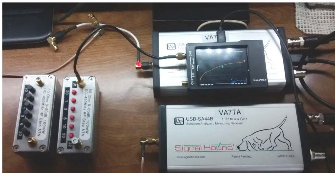
Figure 3 — Signal Hound loss and nanoVNA SWR frequency sweep.
