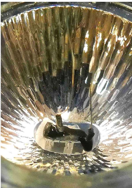
Figure 3 — An exposed filament from a 12 V down light.
