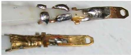
Figure 4 — Spade lug contact mounted on tweezer tips.
