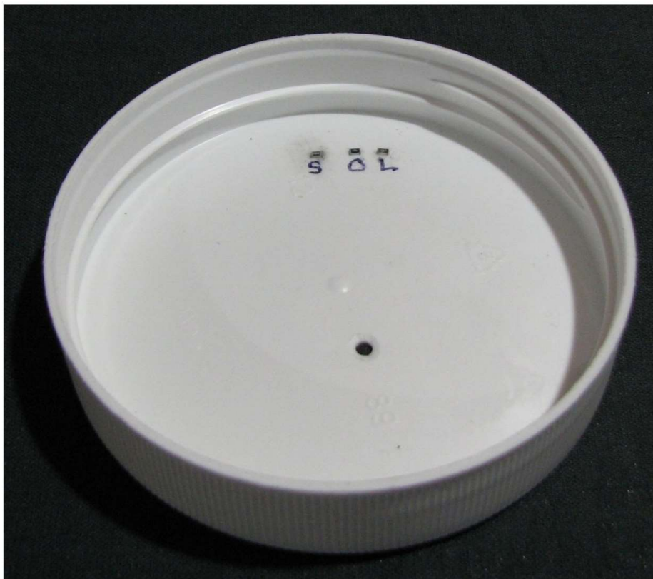
Figure 8 — Loose SMD component measurement tray with initial sol calibration references.
