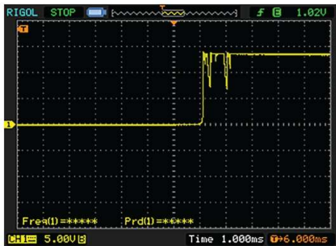
Figure 1 — A sealed relay closes 7 ms after 12 V is applied to its solenoid coil. The 12 V on the moving armature appears at its normally-open port followed by 1 ms of transient noise from mechanical rebound and sliding surface contact.
