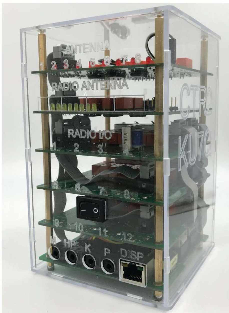
Figure 6 — CTR2 stack with HMI, three RJ45 switch boards, the ASC and the RASC.
