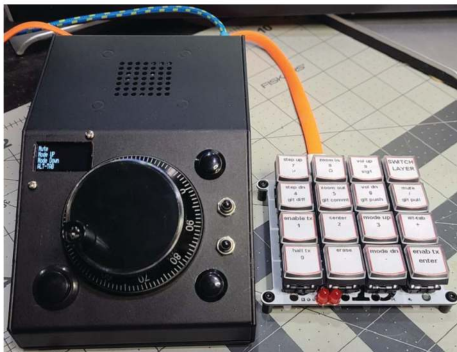
Figure 1 — A rotary encoder (left), and 16 key encoder (right).
