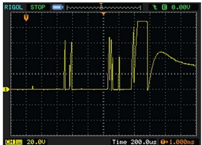
Figure 5 — A sample of the extreme voltages that can occur at the bottom of K2/K3 coil when PTT is released.
