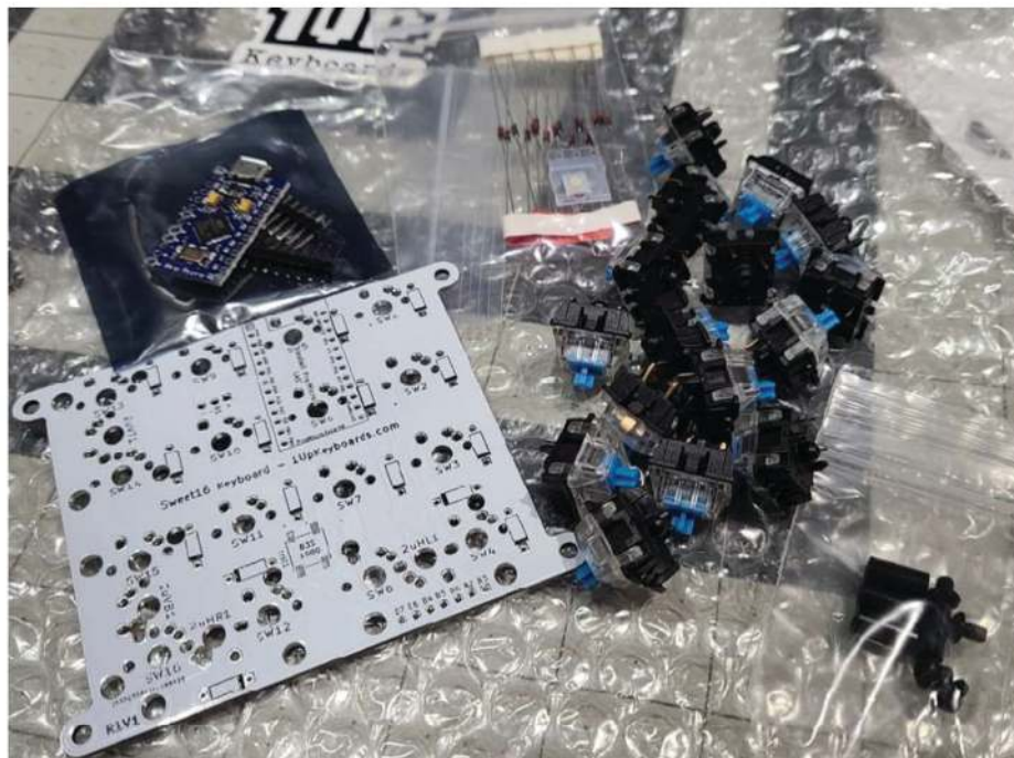
Figure 3 — The components of a 1UP Keyboard kit.
