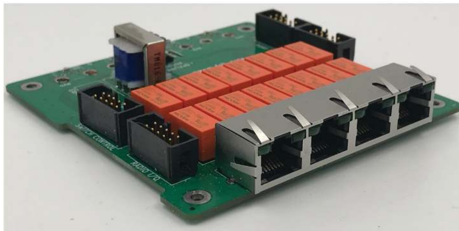
Figure 5 — Close-up of the main 4-port RJ45 switch board.
