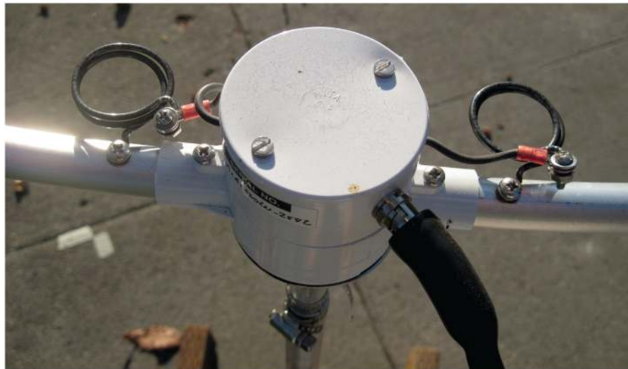
Figure 4 — Inductors inserted between the loop and preamplifier to compensate for the loop inductance reduction caused by the signal amplitude-reducing strap.
