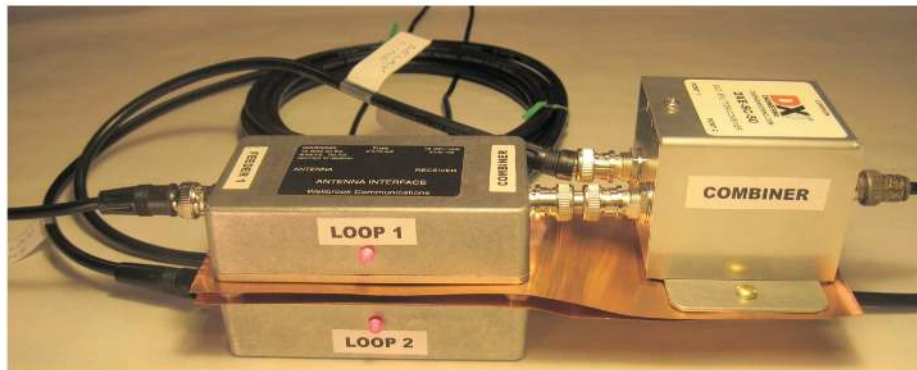
Figure 3 — Antenna interfaces, signal combiner, and delay line.
