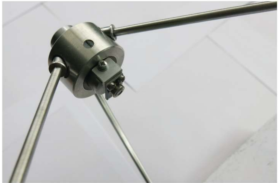
Figure 5 — Melexis sensor mounted at the focus of a 0.46 f/D parabolic reflector.
