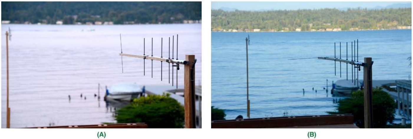
Figure 6 — (A) shows a #12 AWG vertically-oriented wire obstruction mounted to a wooden rod attached to the boom of a Yagi transmit antenna. The receive antenna is 13.4 m away, seen to the left in the distance. (B) shows a horizontal wire obstruction.
