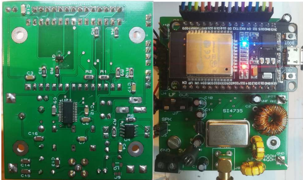
Figure 8 — Prototype SSB receiver board Front (right) and Back (left).
