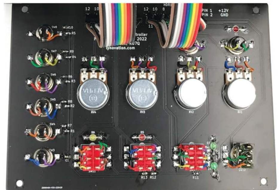
Figure 3 — Bottom of the front panel board showing the design, component wiring, and method of cable management
