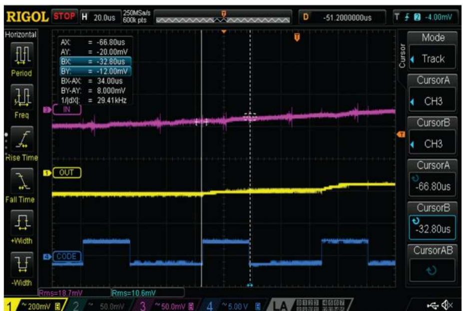
Figure 10 — DSP processing timing signals.
