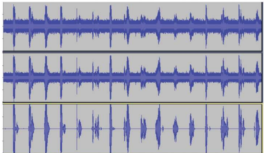
Figure 2 — Audio waveforms with different levels of added noise. SNR from top to bottom: 0.016 dB, 4 dB, and 64 dB.
