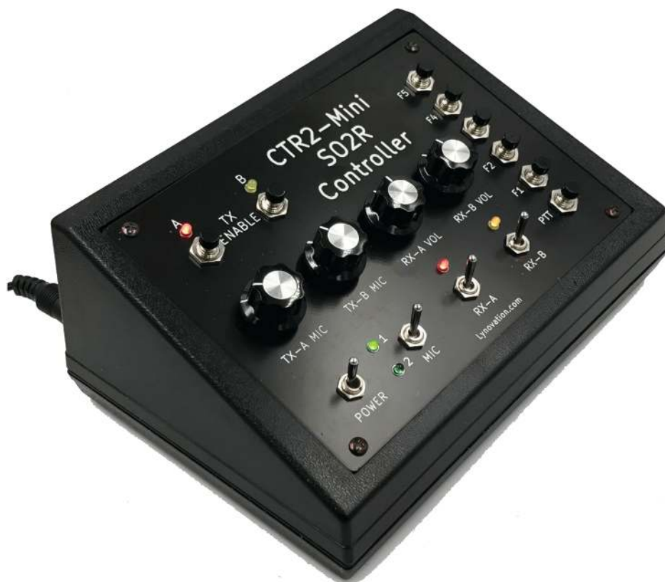
Figure 1 — Completed CTR2-Mini SO2R Controller featuring the PCB front panel created using the techniques described in this article.
