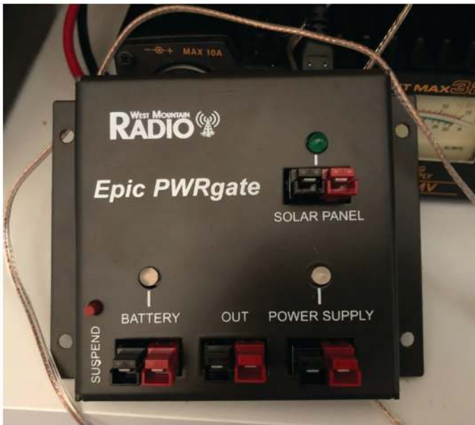
Photo 10 — Epic PwrGate charges the battery and seamlessly powers the system if grid power is lost.
