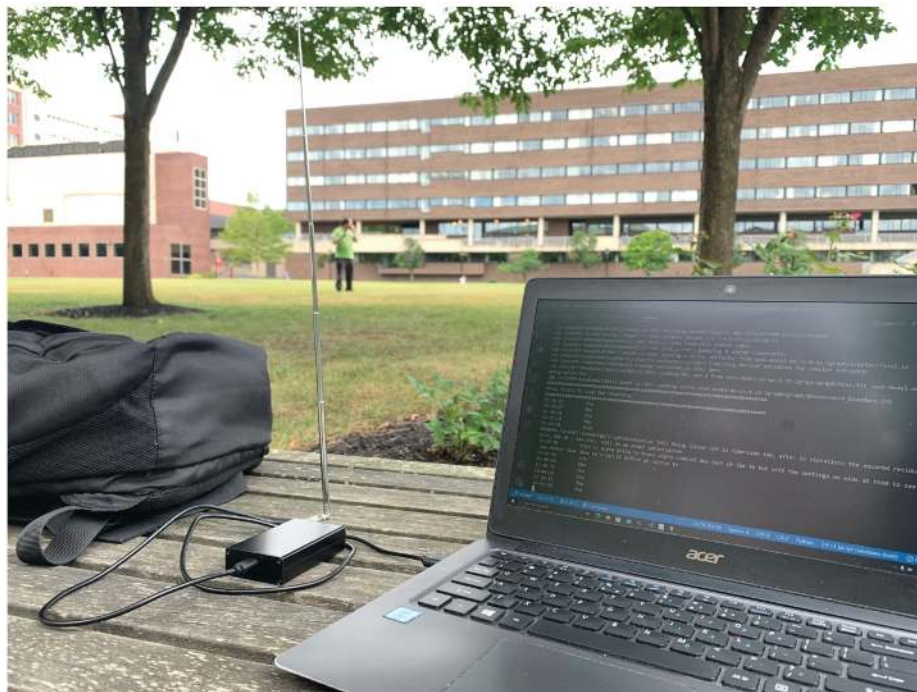
Figure 4 — Brian Callahan, AD2BA, in the background on the RPI campus talking into an HT. You can see the transcription bot in the foreground listening to AD2BA’s transmission and transcribing the audio into text.
