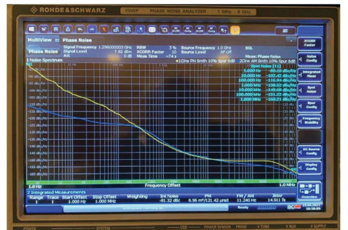
Figure 8 – The currently best possible performance of a 1296 MHz oscillator. This is not a generator using IQ modulators.
