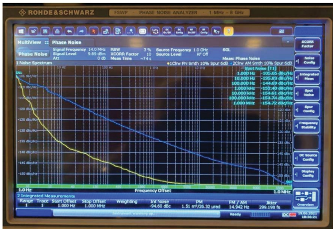
Figure 6 – 14 MHz FM and AM noise plot of a modern digital signal processing based signal generator. Here the yellow line again is the phase noise, that is typically shown in the datasheet, but the high AM (blue upper curve) noise is not mentioned.
