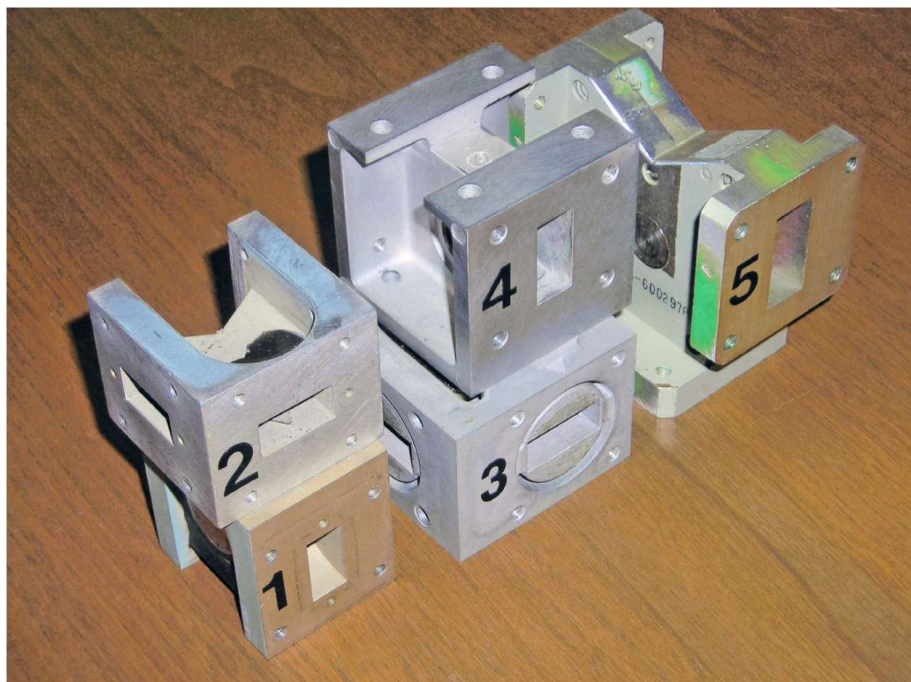
Figure 1 — WR75 circulators labeled 1 and 2 are for commercial satellite television downlinks and digital links. The WR90 and WR112 circulators, labeled 3, 4, and 5, were intended for use on radars.
