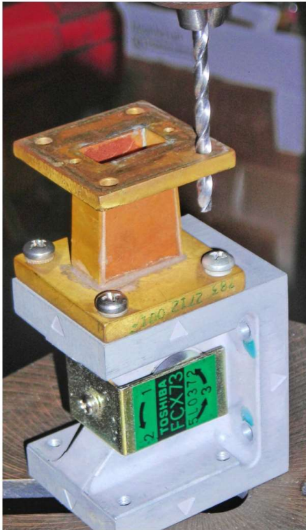
Figure 2 — Clamping or holding everything in position for accurate machining is easy. Flanges can serve as accurate layout guides.
