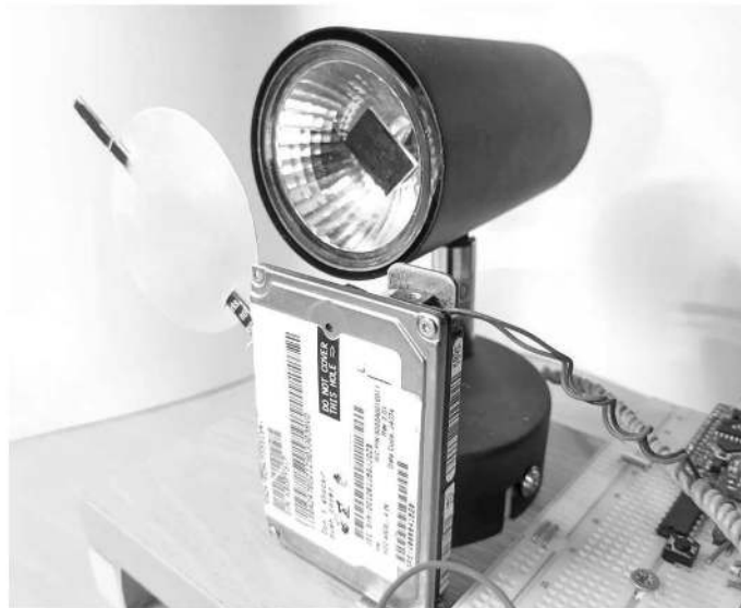
Figure 1 — Heater assembly with paddle mechanical modulator.
