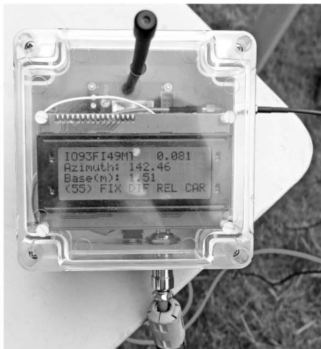
Figure 11 — Rover module and LCD display.
