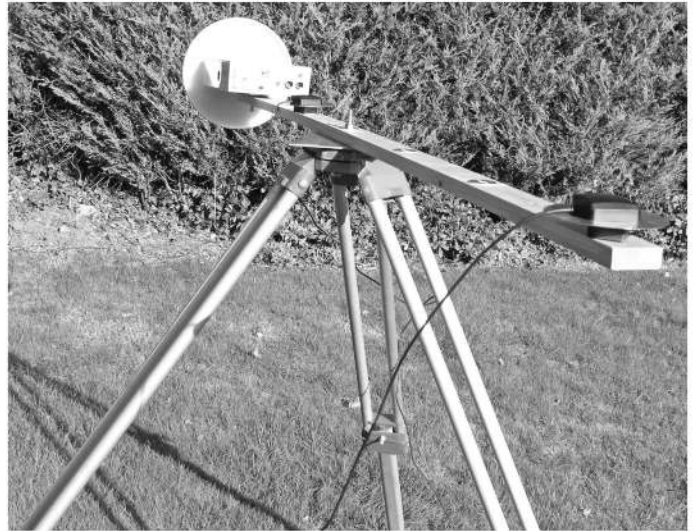
▲ Figure 13 — Rotating baseline parallel to dish antenna aperture.
