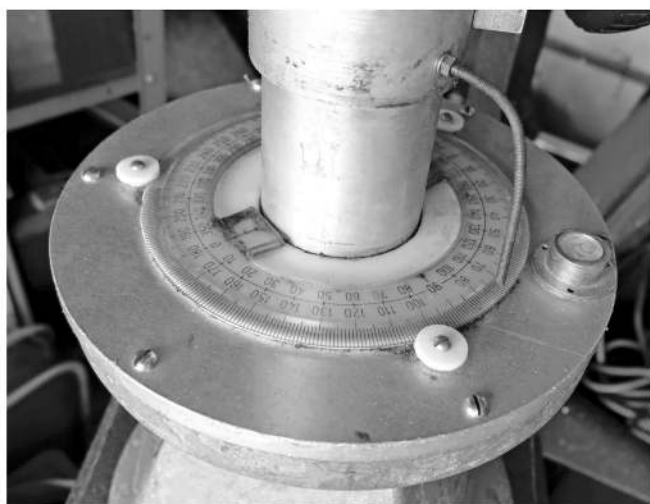
Figure 1 — Rotatable protractor on dish tripod.
