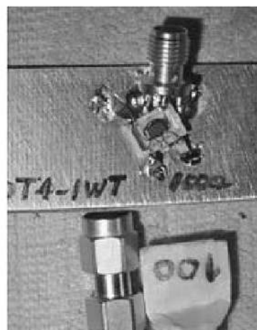
Figure 16 — Winding transformer type MCL ADT4-1WT flipped showing primary and secondary windings.
