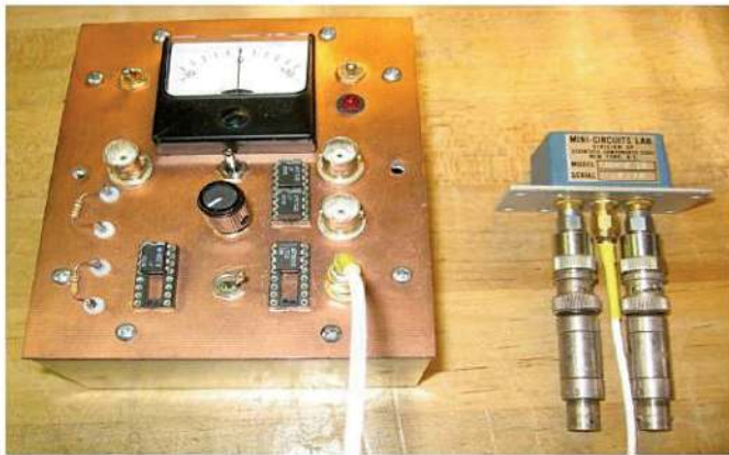
Figure 9 — Phase noise box with DBM. The insulated bushings on the left are tie points for the PLL loop resistors, R2 and R4 in Figure 8.
