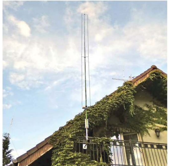
The prototype of the LPi has been built for the 21-29.7 MHz frequency range. Note how small the cross-arms are and how little space this antenna occupies.
