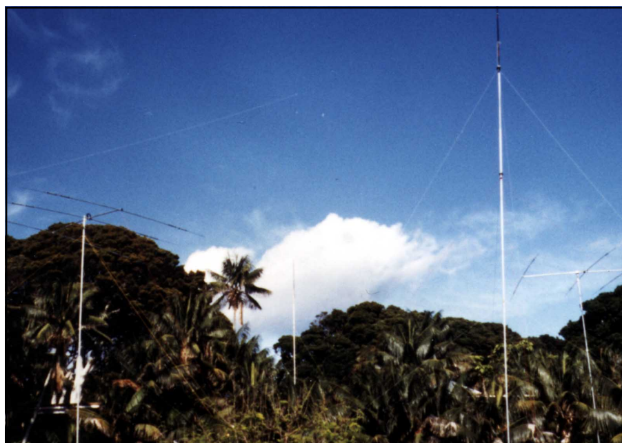
Our low band vertical and two tribanders on the Ebb Tide lawn. Another 40 meter vertical can be seen in front of the cloud; it didn't work well and was removed.
