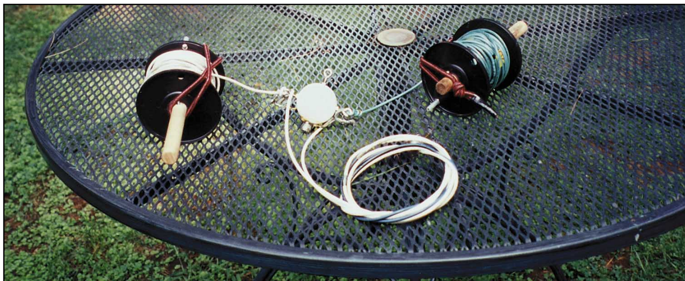
Figure 1—A portable dipole or inverted V antenna. The wire is unrolled from the spools as needed while the rest of the wire remains coiled at the ends. A short transmission-line matching section is connected to the center insulator.
