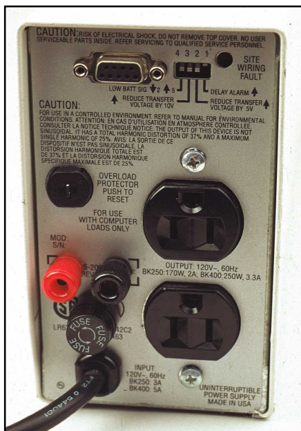
Figure 4—Rear-panel view of a UPS showing an added pair of binding posts and a fuse holder. Carefully position and drill the mounting holes for the added components so that you don't damage existing parts. Ensure the placement of the added components will not interfere with existing parts. A Unibit (see "Tool Tips," Technical Correspondence, QST , Dec 1998, pp 63.) is ideal for cutting through the 1/8-inch thick steel rear panel.
