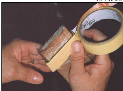
Figure 3—Winding the foil tape tightly on the epoxy-coated paper bobbin on the wooden block. The Mylar tape is unrolled and positioned over the foil layer as you wind.
