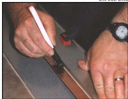
Figure 2—Larry Wolfgang, WR1B, using a 4-foot straightedge designed as a guide for hand-held circular saws to clamp the copper foil tape to a board on a tabletop. After carefully measuring to ensure a uniform 22 mm width, he cut the foil tape using a Fiskars rotary cutter. Be careful to keep the cutter wheel against the straightedge for the entire length. Move the tape in 4-foot intervals to cut the entire length.
