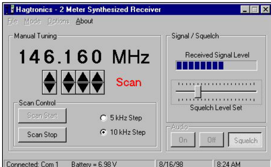
Figure 4—Under PC control, all receiver functions can be controlled via RS-232 commands. Shown here is the manual tuning portion of the PC control program. From this display, the entire receiver can be controlled and the entire 2-meter band scanned. In Memory mode, up to 10 specific user-programmed memory channels can be sequentially scanned. All receiver set-up parameters—such as how long the receiver delays on a scanned signal—can be set for individual users.
