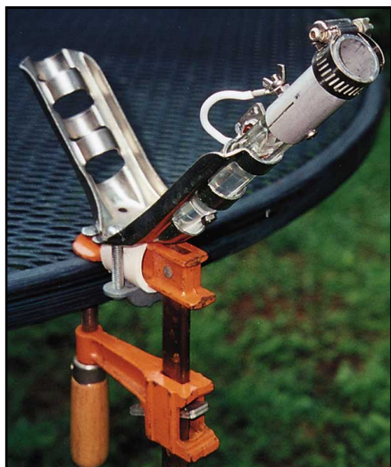
Figure 4—Two flagpole brackets are attached to one bar clamp. One of them must have some of its mounting plate cut away to fit “inside” the other.
