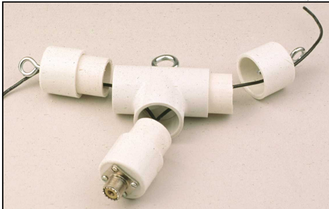
Figure 3 —Group shot of the disassembled pieces showing how they fit together. Short sections ( 1\frac{5}{8} inches) of PVC pipe join the T to the three end caps.
