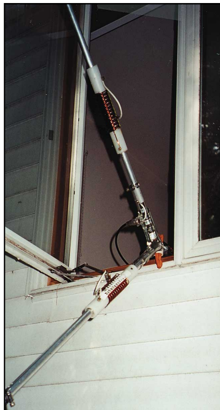
Figure 3—A briefcase portable made from two tubing elements forming a V.
