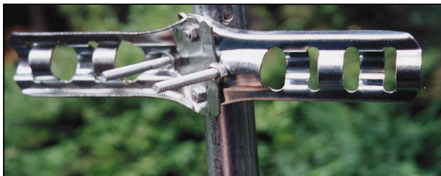
Figure 5—Two tubing elements will also form a dipole when their brackets are bolted together. A U bolt mounts them on a mast.
