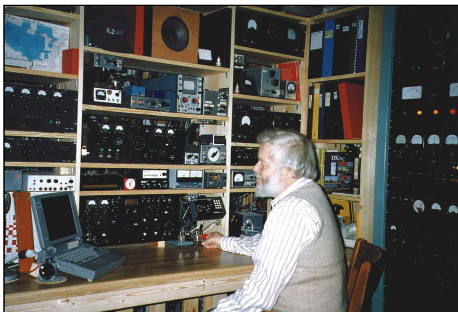
Mark Mandelkern, K5AM, operates on the VHF bands with an entirely home-brew station from Las Cruces, New Mexico. Built over a period of 50 years, the amplifiers run 1500 W on all bands from 1.8 to 144 MHz. The transceiver has special built-in features for weak-signal VHF reception. A complete description of the station appeared in the July/August issue of the ARRL's NCJ: The National Contest Journal .
