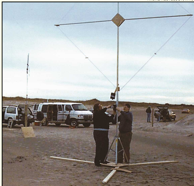
Eight members of AMRAD (the Amateur Radio Research and Development Corporation) journeyed to the wind-swept beach at Nags Head, North Carolina last January to conduct low-frequency listening tests. In the foreground you can see Elton Sanders, WB5MMB and Tracy Wood, K7UO, erecting a low-frequency receiving loop. The small mast in the background supports a remotely tuned e-probe designed by Andre Kesteloot, N4ICK. The AMRAD group used DSP software to monitor signals from Europe (the results were still being analyzed when this was written). During their tests they heard several 1750-meter Lower transmissions from as far away as Pennsylvania. See the AMRAD Web site at http://www.amrad.org .
