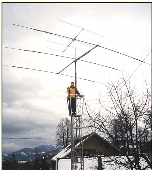
Greetings from Bosnia! Vlado, T97V, maintains an active station in the attic of his home in Vitez. His tower (left) supports a 20, 15 and 10-meter Yagi as well as a 6-meter Yagi. Vlado plans to install antennas for 80 and 160 meters this summer so that he'll be ready for next winter's contest and DX season.
