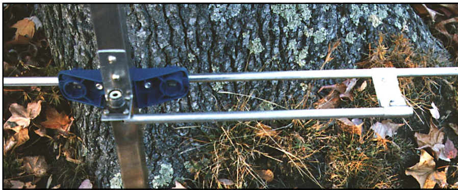
Figure 6—The gamma match and driven element.
