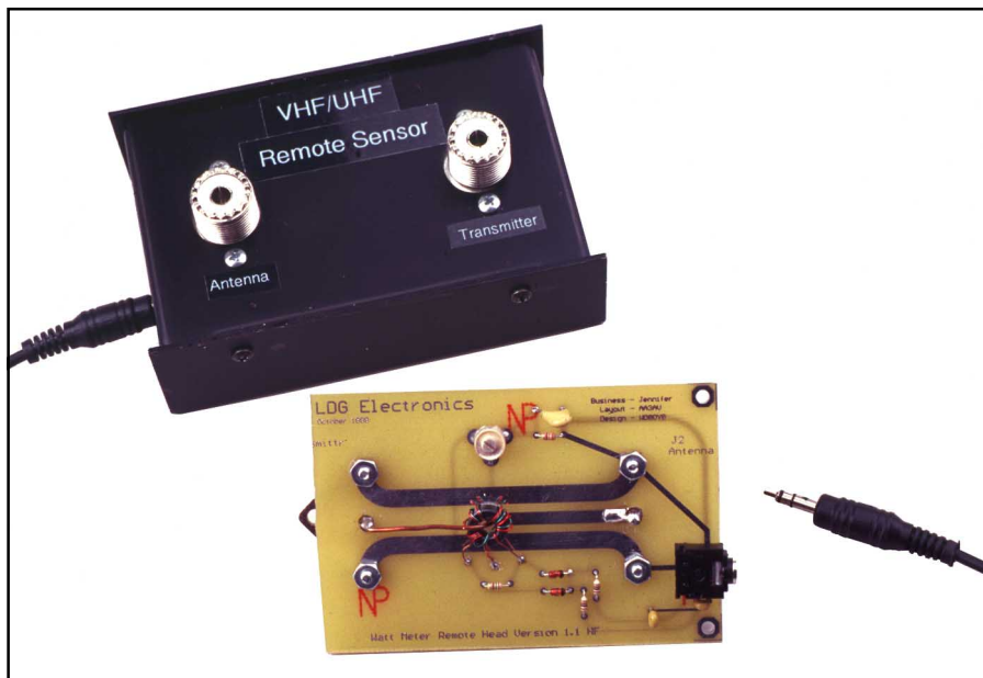
A VHF/UHF sensor inside its enclosure and a rear view of an HF sensor's PC board.
