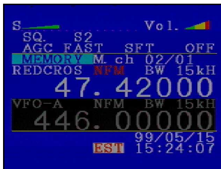
Figure 6—The display screen of the AR7000B showing the contents of memory channel 2 of bank 1. Graphic representations of the signal strength and volume level appear at the top of the screen. The selected squelch level is indicated in S units.
