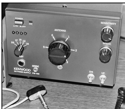
WOFM's custom accessory enclosure: In the center is a six-position rotary antenna switch. Isolooop SENSITIVITY and SPEED controls are at the upper right. The UP and DOWN paddle switches at the lower right are used to adjust the loop to resonance. The loop controller power switch and LED are at the upper left, with the tuning LEDs mounted just below. The loop antenna "band reminder" indicator is at the left center, just above the KEY and 12-V power jacks.
