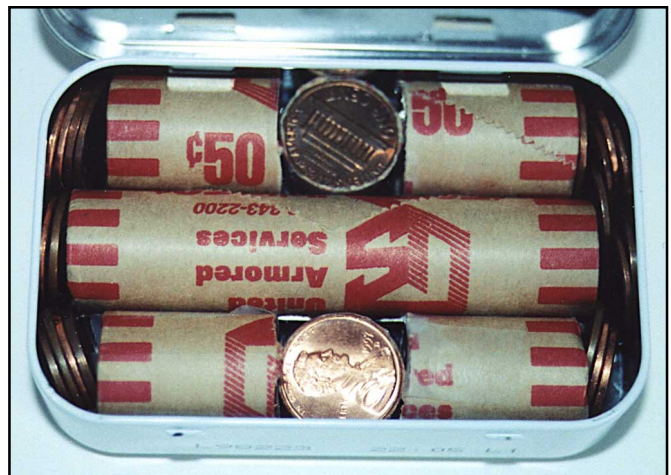
Making the base. Cut approximately 1 inch from each end of two rolls of pennies. Place them in the four corners and stack about eight pennies between them. Fit the third roll into the middle and place the remaining pennies around the sides.
