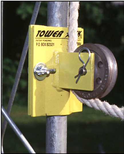
Figure 4—The Tower Block is used on the lifting line of your gin pole. This device allows your ground crew to remain safely outside of the “drop zone.”
