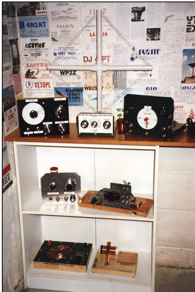
Several homebrew projects dress up the station. Top shelf from the left: 40-meter regenerative receiver 20 using two 3S4 tubes; 40-meter shielded-loop receiver (N1YBT design); 17 and a broadcast-band regenerative using a 1H4G tube. 21 Middle shelf from the left: 40/80 meter regenerative receiver using a 3S4 tube; 22 and a 40/80 meter breadboard CW transmitter (N1TEV design). 18 Bottom shelf from the left: Spider web coil crystal set; 23 and a sliding-inductor crystal set. 24
