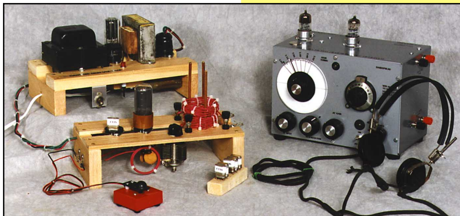
The author’s complete homebrew station on display. On the left is the 6V6 transmitter with its power supply. 12 The two-tube regenerative receiver is on the right.
