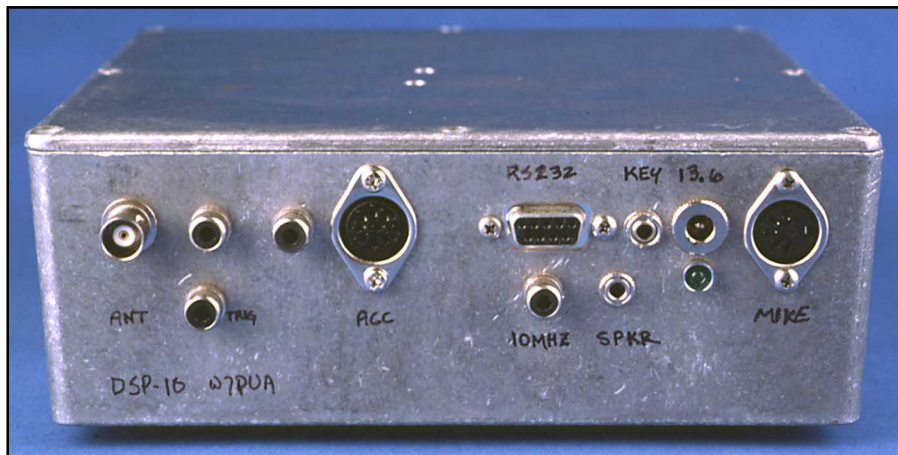
A front-panel view of the transceiver. The two phono jacks adjacent the BNC ANT jack are used for interconnection to an amplifier or transverter. The two jacks can be connected together with a short jumper cable for QRP operation.
