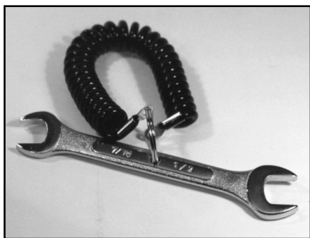
Figure 2—N7CFO's wrist-captive antenna wrench.
