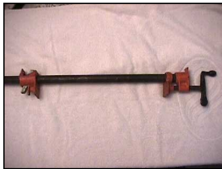
Figure 3—A Pony clamp is familiar to woodworkers and helpful to hams installing towers. Most any moderate-length, medium-duty clamp will work to adjust tower-section fit as described by W1EX.
