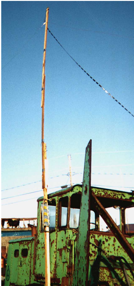
A close-up of our improvised G5RV support mast.
