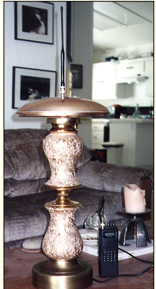
It's a lamp. No, wait, it's an antenna. Jim, N6VNU, is an apartment dwelling ham with severe antenna restrictions. Even taping a 2-meter wire dipole in the window is forbidden. So, Jim Ford, K8ZBA, picked up this lamp at a thrift store for 90 cents, installed an extended "rubber duck" antenna in the top, and discreetly routed the coax through the lamp and out the bottom. When placed near N6VNU's apartment window, it works like a champ.
