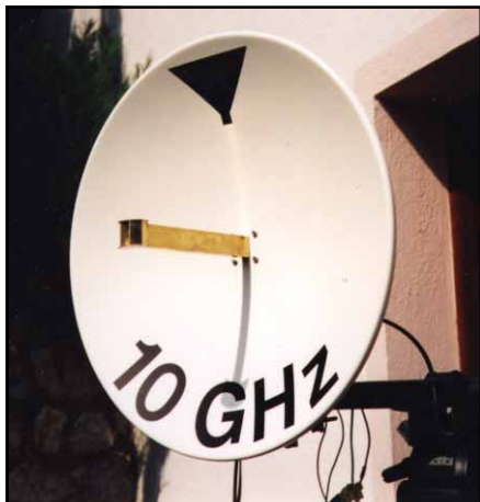
Fig 8—Center-fed Procom dish front view.
