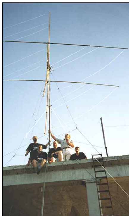
Our 2-element 10-, 15-, and 20-meter quad.
