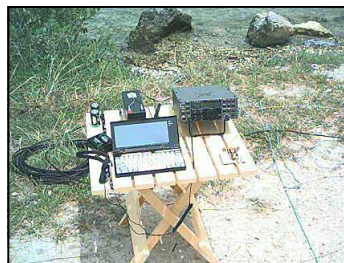
Bob, N4BP's, 'K2 and Poqet computer set up for operating the FOBB from the Florida Keys. This probably well represents the typical setup used in the field.
