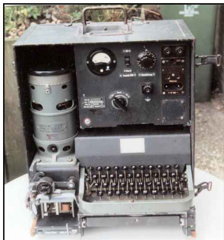
Picture of a 1944 Feldfernsehreiber, thanks to Dick, PA0SE.
