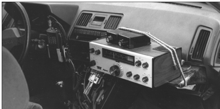
Jeff, AC4HF, operates HF and VHF mobile from his compact car. His Ten Tec Argonaut transceiver handles QRP CW duties, while an H-T keeps Jeff in touch on 2-meter FM. All of the equipment is firmly secured, yet easily removable.
