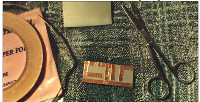
Figure 1—A photo VK1PK's cardboard circuit boards suitable for AF test and experimental circuits.
