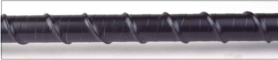
The main shaft of the antenna is wound with a turns spacing of no less than one inch.
