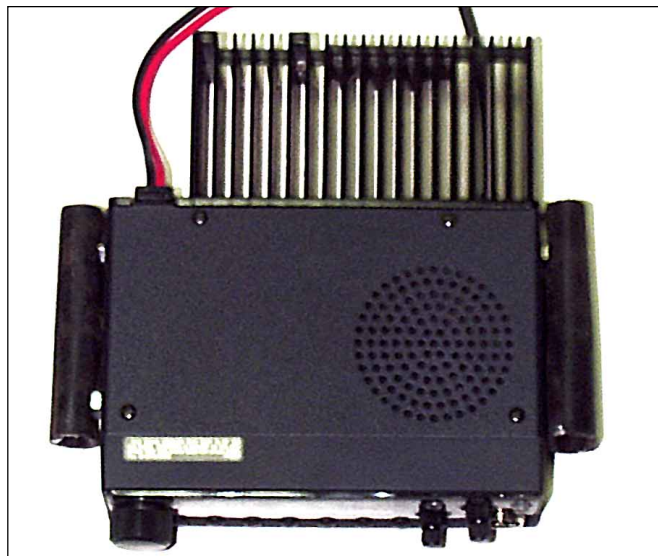
Figure 2—A photo of W5LAN's mobile radio mount, with the hoses on each side.
