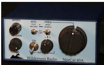
The Wilderness Radio NorCal 40A offers a superhet receiver and 2 W output.
