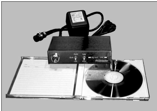
Figure C—The new RIGblaster sound card interface.
