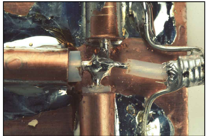
A close up of the T-junction connected to 50-Ω Teflon coax.
