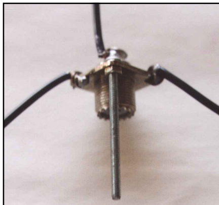
Figure 5—This two-inch screw slips inside the PVC pipe and helps secure the antenna to the flagpole antenna booster.
