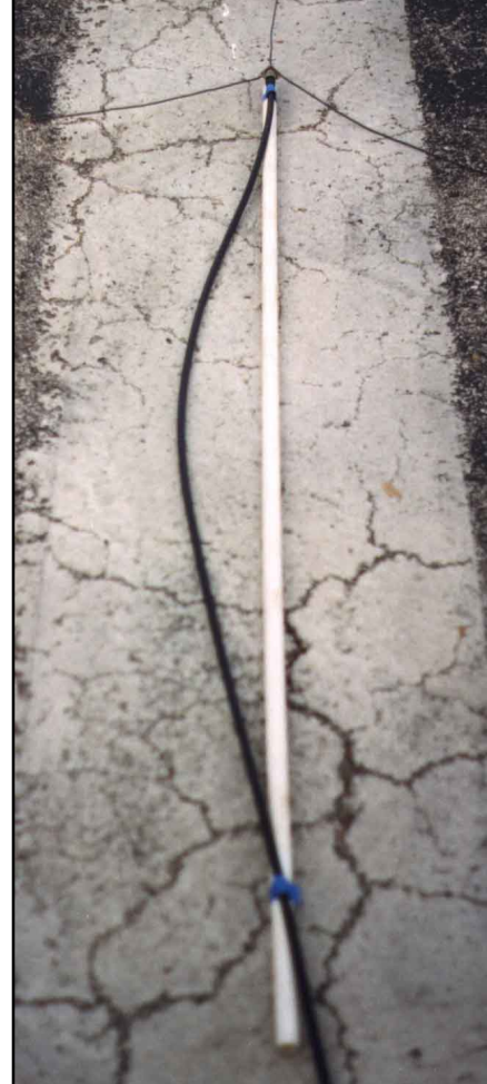
Figure 6—Antenna attached to the flagpole antenna booster, ready to be hoisted. Note the slack intentionally left between the top and bottom tape points.
