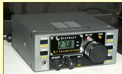
Elecraft's new K1 low-power transceiver, which comes as a kit.
