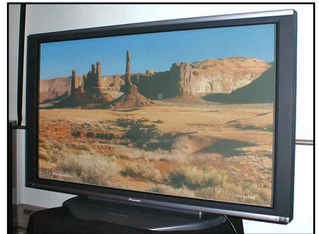
Pioneer's 50-inch plasma-screen TV is only 4 inches thick and weighs less than 90 pounds. It can be used to show DTV and HDTV signals.
