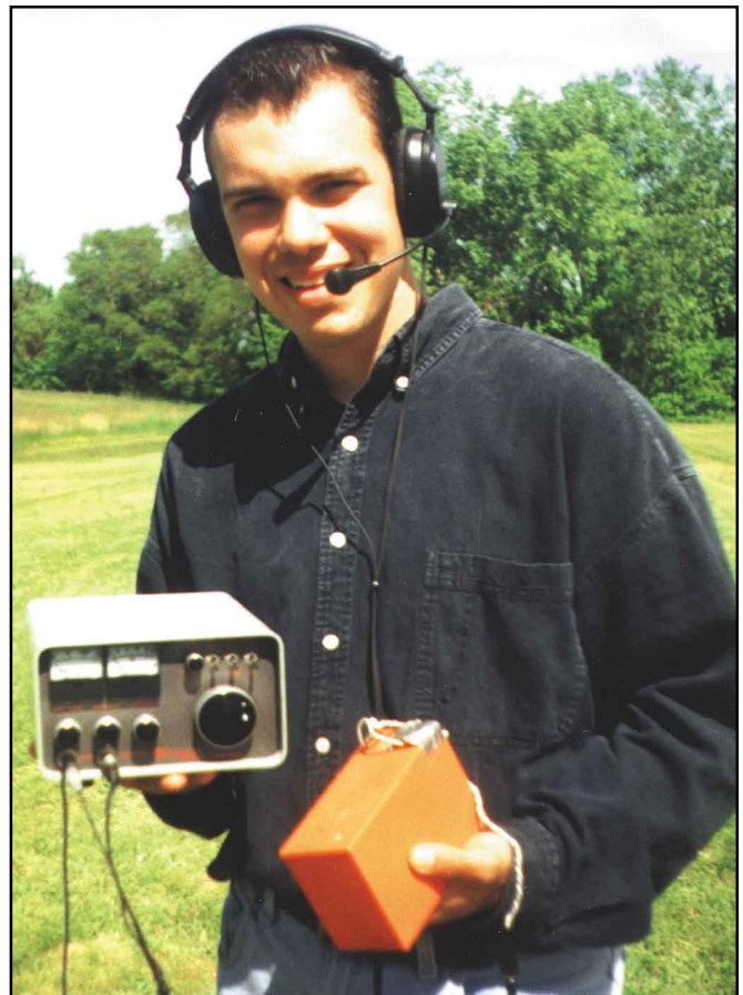
The author enjoys working the microwaves with a portable 10-GHz Gunnplexer transceiver.
