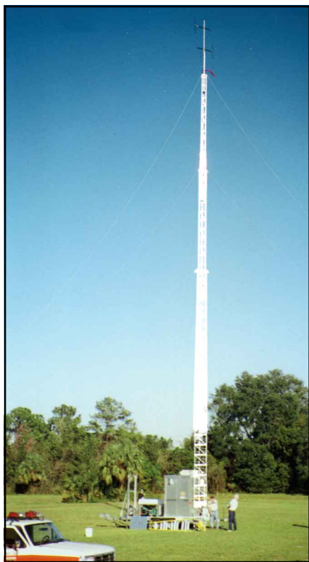
Seminole County, Florida, ARES/RACES members trained as a deployment team under the Department of Forestry with this transportable Mutual Aid Communications Unit with 100-foot crank-up tower, generator, and shelter for VHF and UHF base radios and hand-helds.
