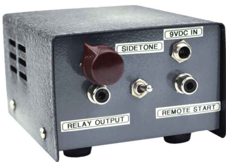
At the top left of the rear panel is the sidetone level pot ( SIDETONE ). S2, the sidetone on/off switch, is in the middle of the panel. J1 ( REMOTE START ), J2 ( RELAY OUTPUT ) and J3 ( 9V DC IN ) fill the remainder of the panel.
