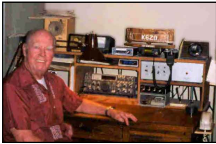
Ed, K6ZO, has a modest setup including a Kenwood TS-930S, homebrew 4-1000 amplifier and a 4-element 20-meter monobander up 60 feet.
