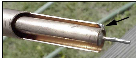
Figure 9—This cutaway view shows the tabs of the Q section and lower element soldered together.
