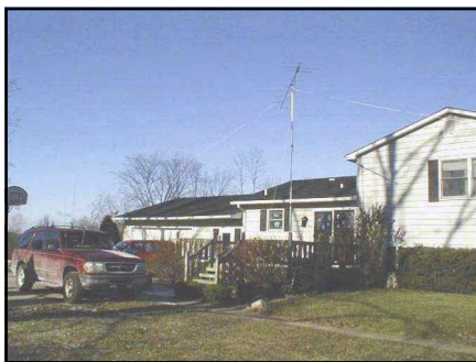
An 11-element Yagi on telescoping paint pole for portable operation at our son Steve's home near Clio, Michigan.
