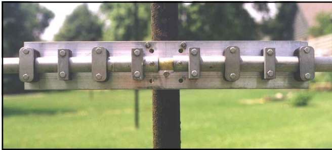
Figure 4—The strengthened antenna mounted on my improved mounting assembly.
