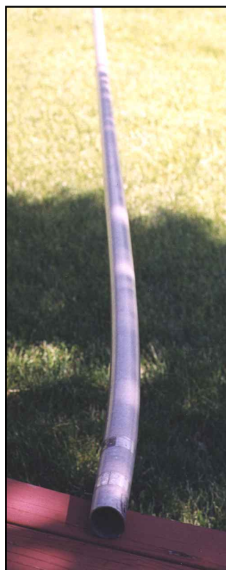
Figure 1—This bent tubing at the center mounting plate resulted from a windstorm.
