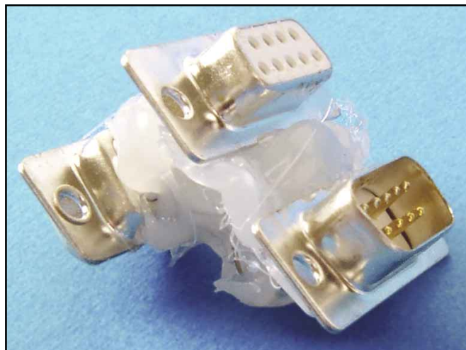
Figure 3—This simple Y adapter consists of one female DB9 socket interconnected with two DB9 male jacks, all held together with noncorrosive sealing compound.
