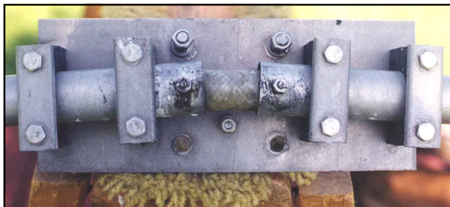
Figure 2—This extreme distortion where the tubing attaches to the mounting plate is ominous.
