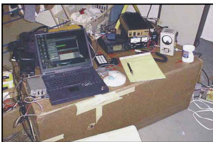
The “basement-portable” operating position at Clio, Michigan. The hardware includes an IC-706 MKII transceiver, 150-W amp, MFJ switching power supply, Bird wattmeter, GW2K laptop computer running WinMSDSP, audio filter and coffee cup! Notice the very fancy recycled cardboard box operating table they gave me!
