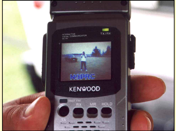
A hands-on demo. W9ZL, the Fox Cities Amateur Radio Club, used a Kenwood VC-H1 to demonstrate slow-scan television.
