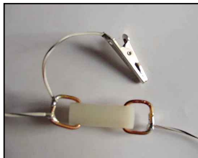
Figure 2— The band switches are constructed from nylon spacers, some wire and an alligator clip.
