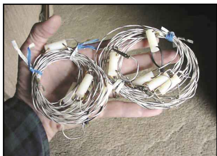
The entire antenna can be collapsed to a size that fits in the palm of your hand!
