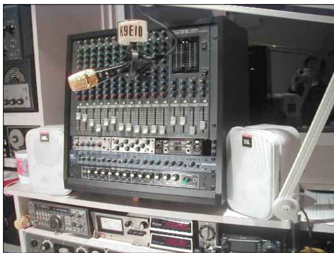
Fig 2—An audio rack at my station. Equipment is as follows: (top unit, including row of slider pots) INTER M Model 1242 12-channel mixing console; (second row, three units) SLM Model SM4CL compressor/limiter, SM3PE three-band PARAMETRIC EQ and CBL cable doctor patch bay/ cable tester; (third row) SYMETRIX Model 528 microphone preamp/ processor; (fourth row) Heil Sound Model 435 four-band parametric equalizer. Also in photo: Heil Sound Model GM-5 GOLDLINE microphone; Luxo Model LX-1 microphone boom; AT-1 Model SM-1 microphone shock mount.
