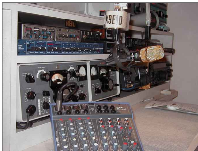
Fig 3—Equipment in my shack: (top row, three units) SM3PE three-band PARAMETRIC EQ, SLM Model SM4CL compressor/ limiter and a homebrew patch panel; (second row) SYMETRIX Model 528 microphone preamp/processor; (third row) Collins KWM-2A/312 B-5 (on desk) SPIRIT four-channel mixing console.
