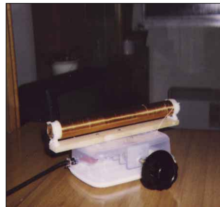
Fig 7 —G2BZQ's completed Giant LF loopstick antenna.
