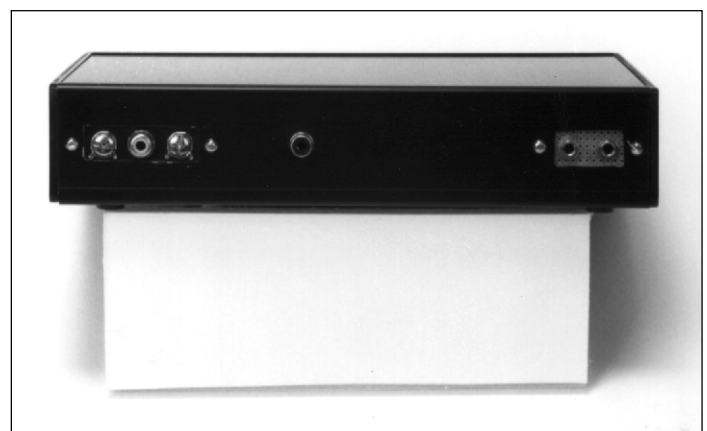
Fig 10—Rear view showing, from left to right, combined J201/TB201 (input from DDS/TR from HW-101), J202 (VFO out), J203 and J204 (dc power from wall adapters).
