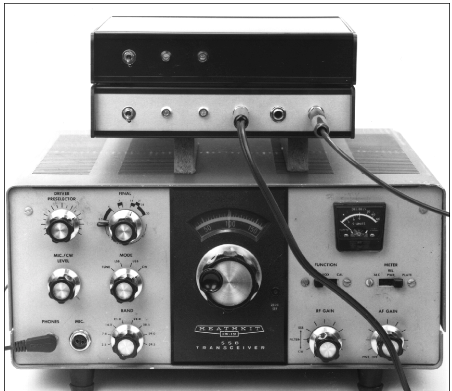
Fig 7—PLL unit atop matching DDS unit, with HW-101 HF transceiver below. On PLL unit front panel, from left to right, S101 (power switch), D101 (red POWER LED indicator) and D102 (green PLL LOCK LED indicator).
