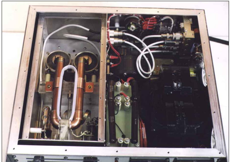
Fig 1 —A top view of the amplifier. The plate transformer in the front right and high-voltage power assembly next to it occupy the majority of the control side with the blower, filament and control transformers sitting just behind. The tank compartment with the cover removed shows the plate line on its Plexiglas stand.
