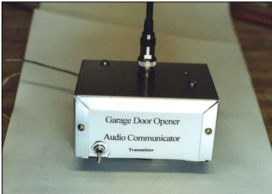
Fig 3—The audio garage door opener. Above, the transmitter module is on its own board and inserted into halves of a DIP socket (upper left center). The microprocessor and multiplexer are DIP ICs surface mounted to a copper-clad board (right center). Four NiCds are in a dark bundle to the right. Below is the finished product with a BNC connector and commercially made \lambda/4 antenna. The BNC allows for future antenna experiments.
