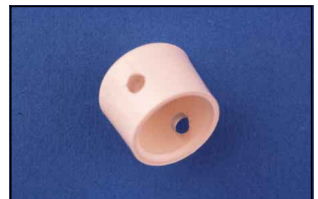
Fig 4—A machined CPVC pipe cap showing the carved hole (lower).
