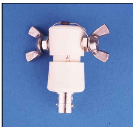
Fig 7—The completed balun with a 200-Ω 1/4-W carbon-composition resistor used for return-loss measurements. The balun is in a typical mounting position, with the load resistor across its top.
