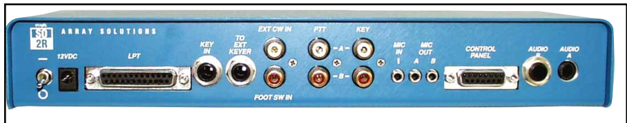
Figure 2—The rear panel of the input/output box.
