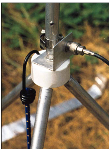
Figure 1—The top of the tripod with the bottom section of the mast connected to it. A bolt holds the three leg supports in the PVC cap slots. This bolt also passes through the 1\frac{1}{2} \times 1\frac{1}{2} -inch aluminum-angle piece that supports an SO-239 chassis connector for feed-line connection. A \frac{1}{4} -inch hole in the cap top accepts the bungee-cord hook.
