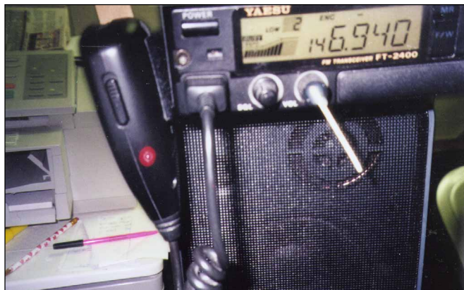
Figure 7—W1HQ's 2-meter transceiver with several modifications to aid those with poor muscle control. The PTT paddle is on the far side of the mic. The red LED is visible on the mic's near side. Hook-and-loop material secures the mic on the side of the radio, and a toothpick makes the volume control more manageable.
