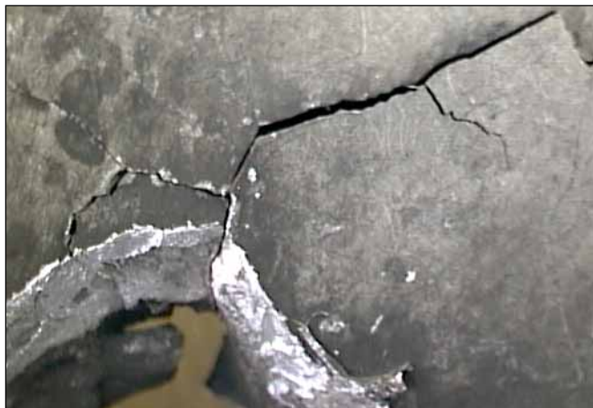
Figure 5—A close-up view of cracks in the failed mounting plate.
