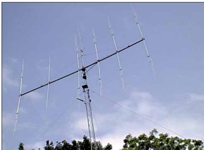
Figure 6—KC5UH's KT-34A hangs on its truss wires after the ancient mounting plate failed.
