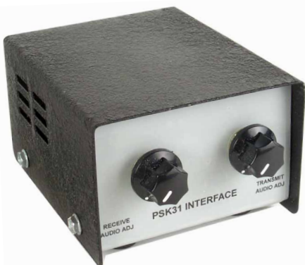
Figure 2—For the front-panel labeling, Rick used a 2x4 1/8-inch clear Avery shipping label (#5663) made for use with a LaserJet printer. These labels are available at Staples and other office-supply stores.
