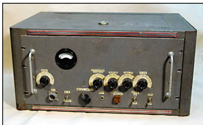
A view of the entire converted BC-625 in its Bud cabinet.
