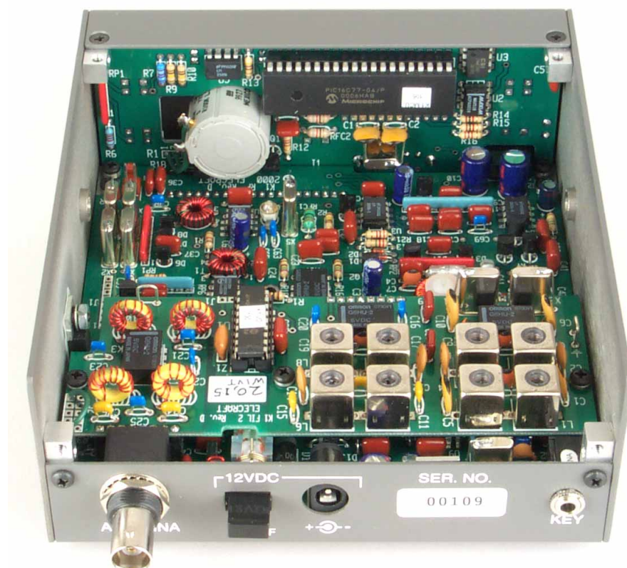
Figure 3—An internal view of W1VT's K1. The Front Panel Board plugs into the main board along its front edge. The Filter Board, which determines the two bands covered by the transceiver, is towards the rear of the enclosure (the foreground in this photo). It's positioned above the RF Board and connects to it through three 8-pin headers. Three small screws secure it in place.
