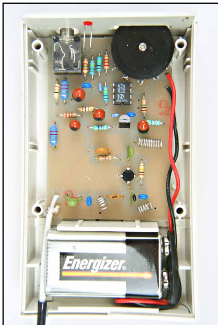
An inside view of the neatly assembled TRF RFI receiver prototype.
