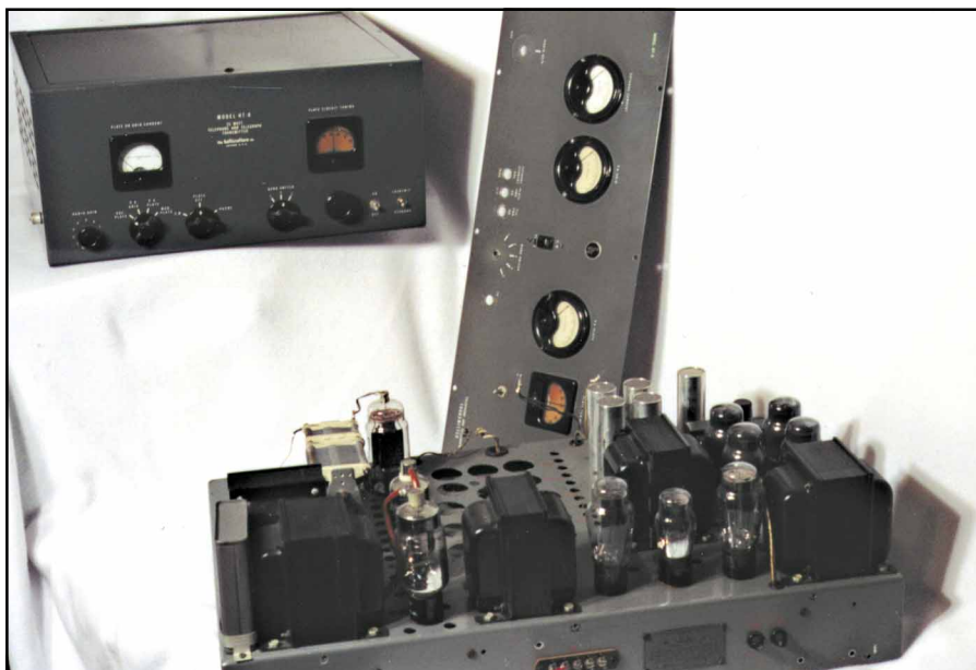
A Hallicrafters HT-9 (foreground) in the process of being restored, with its little brother, the HT-6, in the background.
