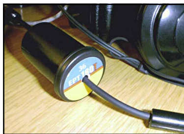
Figure 3—K4NR housed the isolation transformer in a film can with the connections made through two-conductor plugs and jacks on “pigtails.”
