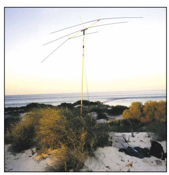
Jack set up his portable Yagi on the beach at Monkey Mia on Australia's West Coast. A PVC joint slipped, causing one of the elements to twist out of alignment. No matter, as VK1XQ worked 30 JAs with his 1-W hand-held from this location.
