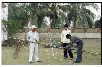
Setting up the ground-plane and five-element Yagi antennas built by VU3BIS.
