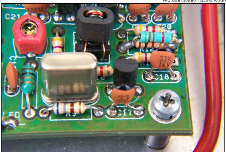
Figure 2—Change the value of R12 to approximately 330  $\Omega$  by placing a 500- $\Omega$ ,  $I_8$ -W resistor (R12A) in parallel with the original 1-k $\Omega$  resistor. C17 and C18 are also shown here.
