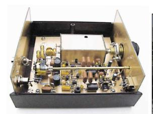
**Ugly construction? No way!** Denny Payton, N9JXY, built this version of the Binaural IQ receiver by Rick Campbell, KK7B (see the March 1999 *QST*, page 44). Denny used the ground plane technique (sometimes referred to as "ugly construction"), but went to great pains to keep the leads straight and the soldering perfect. The result is a 40-meter receiver with remarkable performance.
