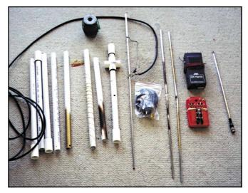
The complete VK1XQ portable 6-meter station, with coax, PVC boom sections, telescoping Yagi elements, the AEA Handy, a keyer (almost as big as the rig), and telescoping whip fits neatly in a small pack.
