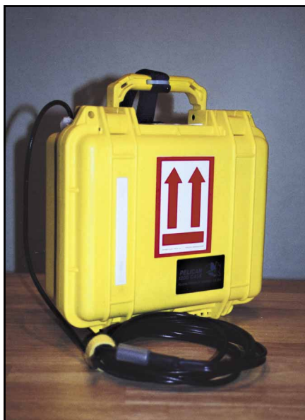
The APRS tracker units sent aloft with the Challenge balloons.
