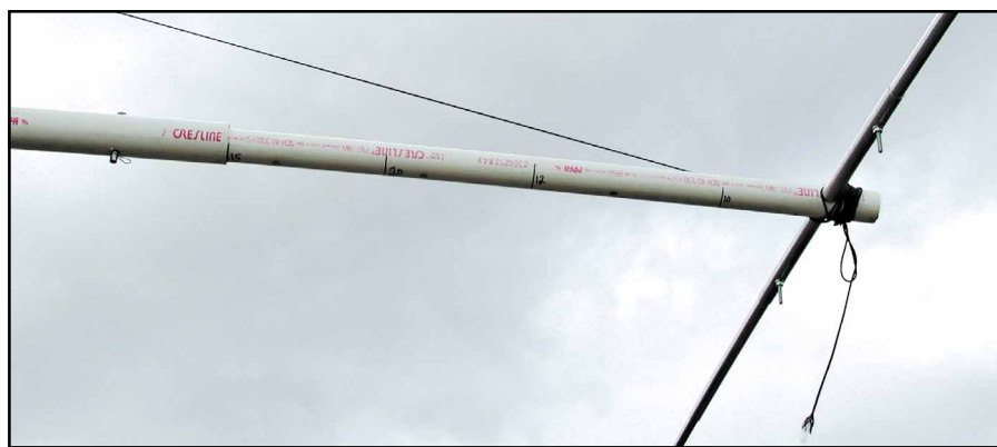
This view illustrates how the director attaches to the telescoping boom.
