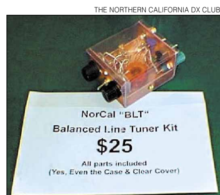
Figure 3—The NorCal BLT, a Balanced Line Tuner designed for QRP operation in the field.
