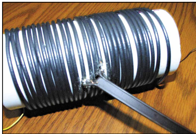
A close-up view of the feed line/coil connection.
