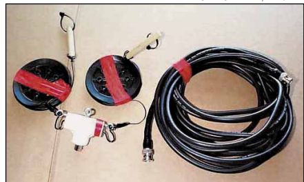
Figure 1—This 40 meter Appalachian Trail dipole from the EPQ-QRP Club is fed with 50-ohm RG-8X coaxial cable.
