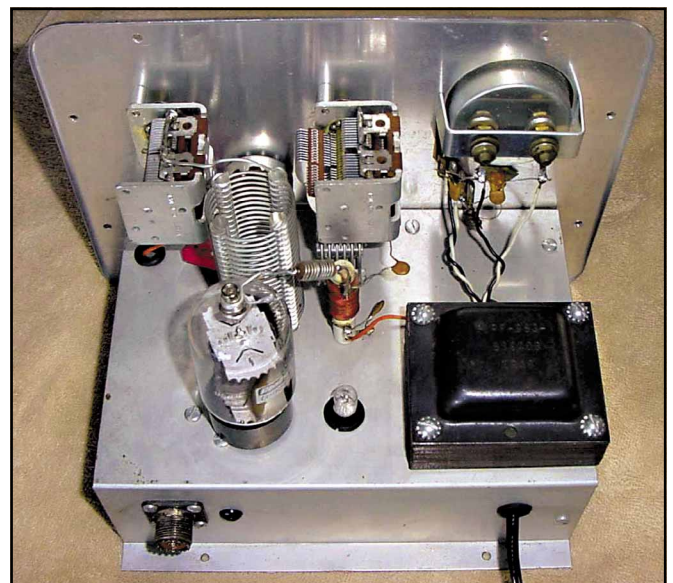
The clean interior layout of the 400 transmitter.
