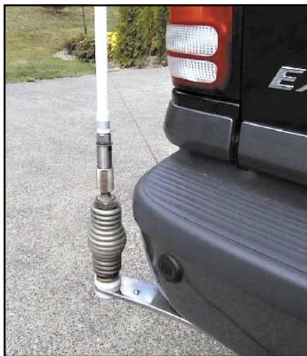
The sturdy antenna mount crafted from a stainless steel bar.
