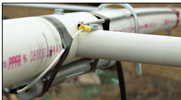
A detailed view of the hairpin match and balun assembly.
