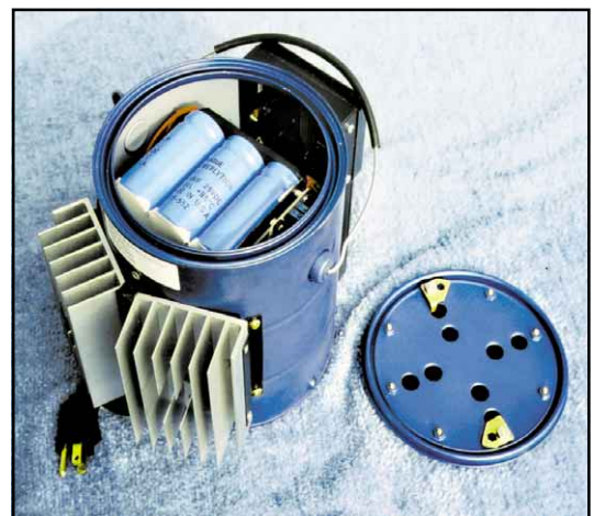
"Can" do! Phil Caubarreaux, KB5EKD, opted to build a 20-A, 13.8-V dc power supply into a paint can (top). The heat sinks mount on the opposite side from the meter and connection posts (bottom).
