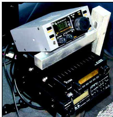
Figure 1—My QRP sandwich: Elecraft K1 at the top, ICOM 2-meter transceiver in the middle, attached to a RadioShack scanner.
