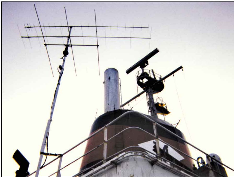
Clint Walker, W1LP, is captain of the Chemical Pioneer , which makes it convenient for him to mount 50, 144 and 432-MHz Yagis on the railing of his ship. Other antennas, including the ship's long wires and one for radar, can also be seen in this view.
