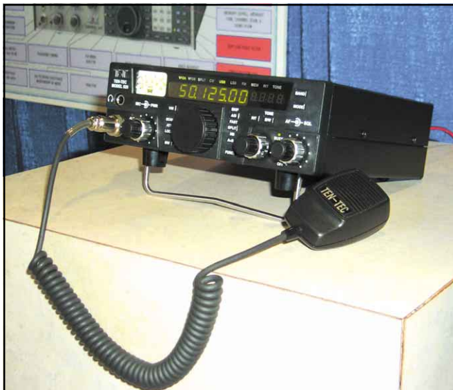
The Ten Tec 6N2 all-mode 6 and 2-meter transceiver. It offers extended FM receive from 136 to 174 MHz, separate output connectors for each band, and a transverter port.
