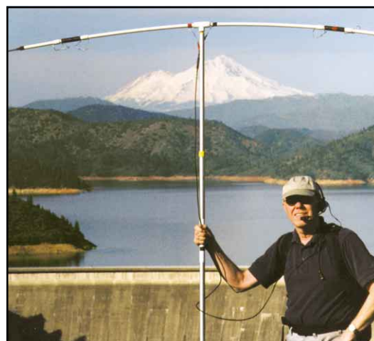
A ramblin' man. Budd Drummond, W3FF, has been walking and talking with his backpack station since January 2000. So far he has worked all US states and Canadian provinces, along with more than 120 DXCC entities. Budd's pedestrian portable operation consists of a 5-band dipole, a Kenwood TS-50 transceiver and a 4-pound sealed lead acid battery. This photo found him in California with Mt Shasta looming in the background.
