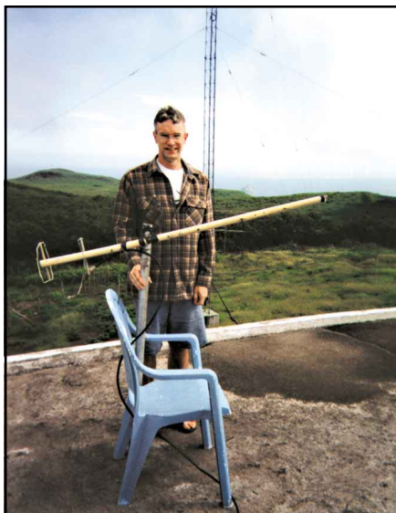
The author and the quagi uplink antenna (aimed at OSCAR 10). The blue chair is the official "stabilization unit."
