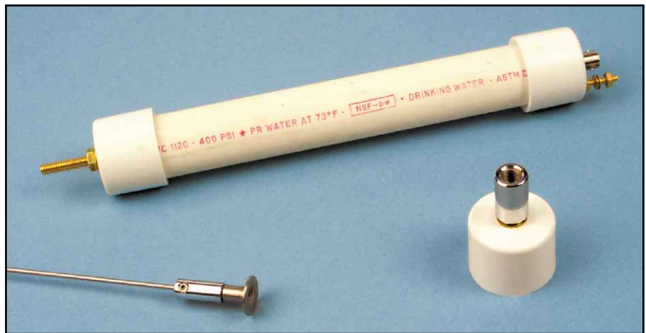
The active antenna is housed in a Schedule-40 PVC tube with connections at opposite ends for the whip antenna element and the coaxial cable to the power supply and receivers.
