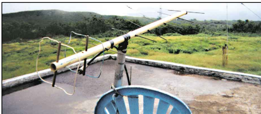
A close-up view of the homebrew quagi used for the HC8N satellite uplink.
