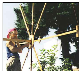
Figure 7—At left, a cedar version of the 20-meter Double Cross quad at VE7FJR just before it was installed. Above, Dave, VE7DWG, assembles the quad elements to the boom.
