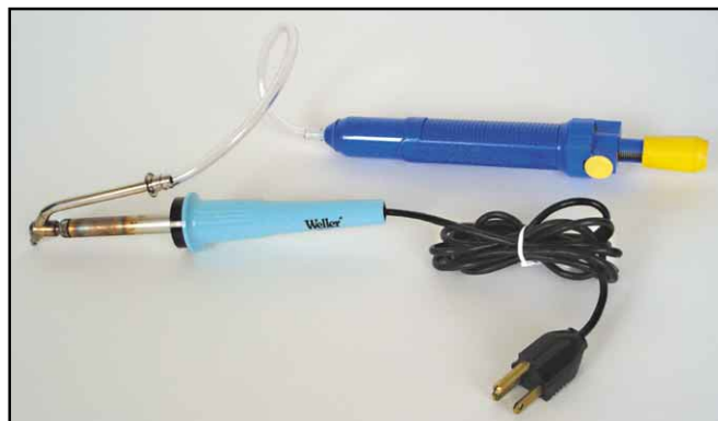
Figure 1—KC1SX's custom desoldering tool.
