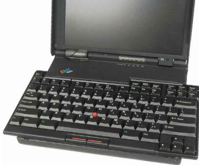
The IBM 701C "Butterfly" (486 with decent sound hardware) has what is arguably the niftiest keyboard ever to appear on a laptop. When the lid is closed the keyboard folds in on itself like a collapsing Tetris puzzle and does not extend beyond the edge of the laptop (as it does when it's in use).
