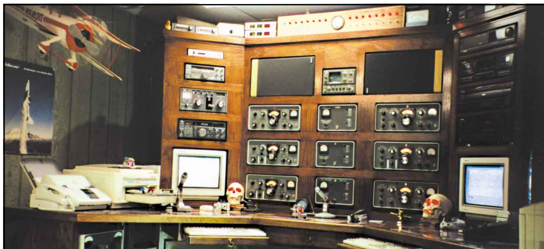
Console yourself— Norman Wolfe, KL7IVK, of Fort Atkinson, Wisconsin, did, and here are the results! His Collins gear (only): 75S-3B receiver, 75S-3C (he's got two of them), 312-B4 station console (three), 32S-3 transmitter (two), 32S-3A transmitter and 30S-1 linear.
