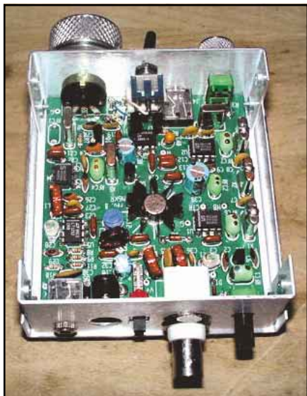
The SST-20, with the dual varactor diodes and switching arrangement visible—before the K1EL keyer module was installed.
