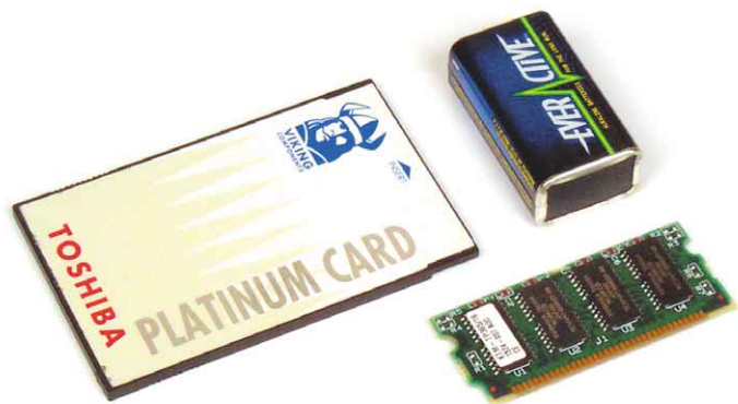
Laptop RAM, old and new. Shown here is credit card RAM from the mid-’90s and a more recent SODIMM module on the right.
