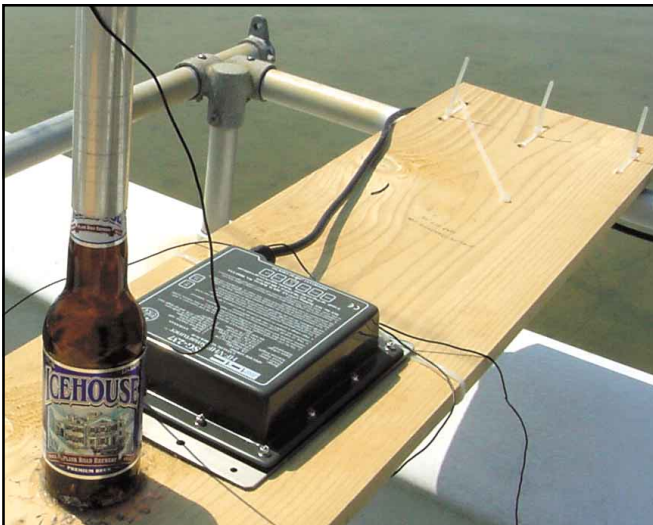
Details of the base insulator and tuner of N4RNM's vertical cat antenna.
