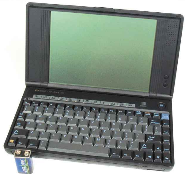
This HP Omnibook 300 is more of a palmtop than a laptop. The tiny precursor to today's Windows CE machines has its software and operating system in ROM cards. It's a cult classic—something to be collected just for the fun of it.
