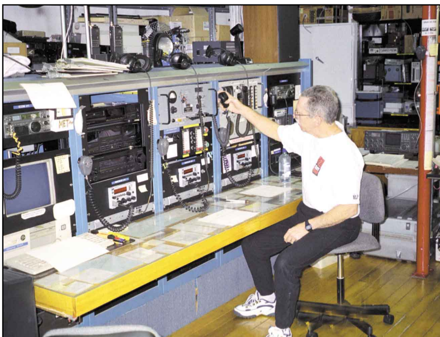
Figure 6—South Pole Communications Center with Neil Conant, N8BPR, at the console. All station HF and VHF communications originate here.
