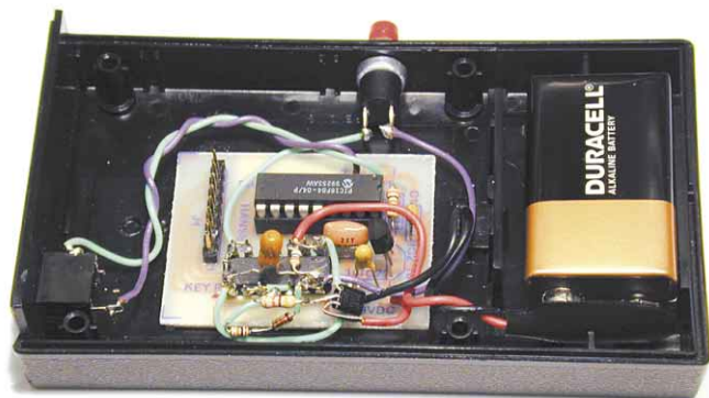
Figure 3—The battery-saver circuit installed in a shack accessory.
